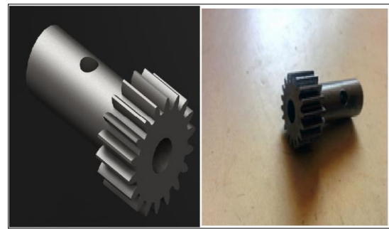
Figure 5: Pinion Gear - CAD model and the manufacturing component
