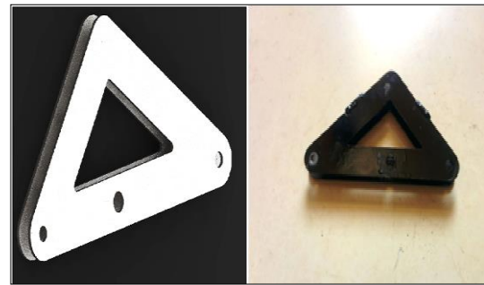
Figure 3: Rocker Arm - CAD model and the manufacturing component
