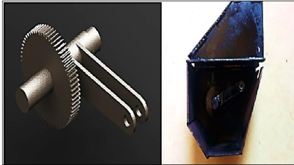
Figure 4: Wheel Gear Assembly - CAD model and the manufacturing component.
