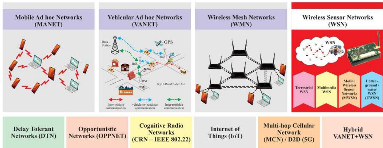
Fig. 1 Sub-domains of Wireless Multi-hop network
