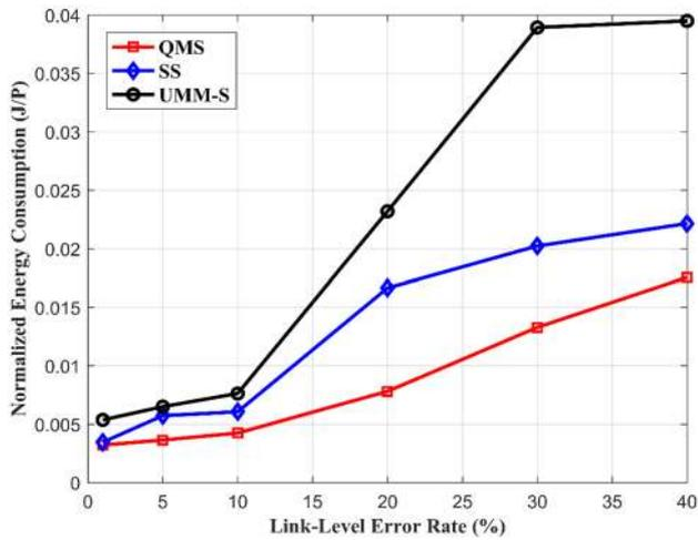
Fig. 16 Normalized energy consumption (J) vs PER (link-level)
