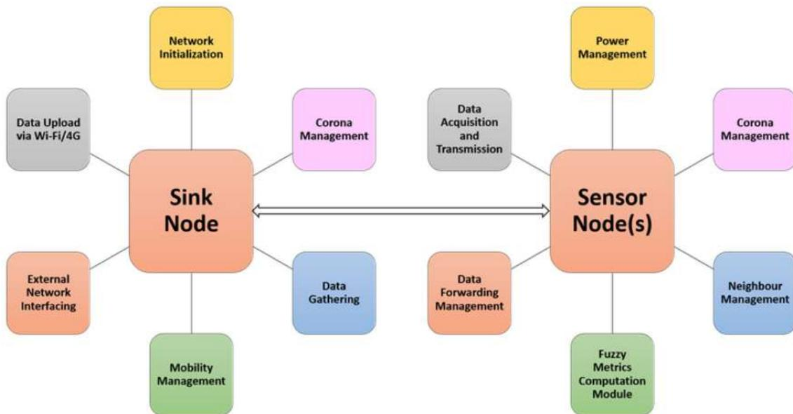
Fig. 2 Sink and sensor node(s) functionalities in WSN
