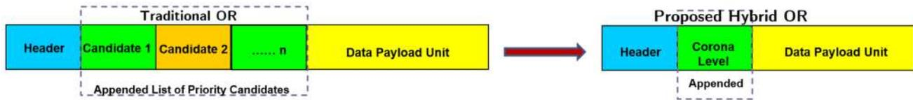
Fig. 5 Packet header—proposed hybrid OR
