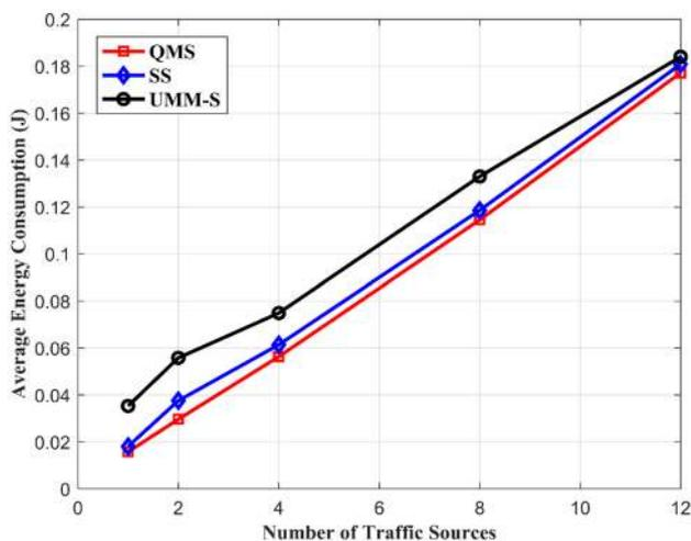
Fig. 11 Average energy consumption (J) vs Traffic sources
