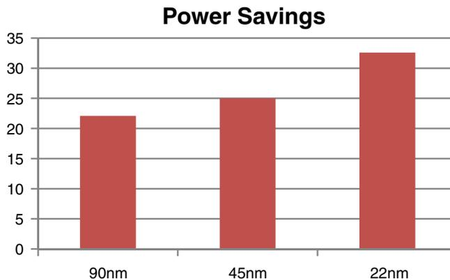
**Figure 6.** Power savings of 3T NAND gate.
