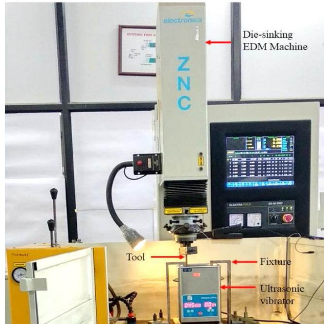
**Figure 1.** Experimental setup for powder mixed Electrical discharge machining.
