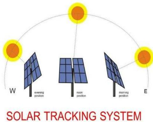
**Figure 2.** Solar Tracking Mechanism
