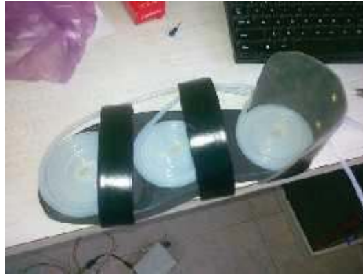
Fig. 1. Model of shoe with three air bladders
