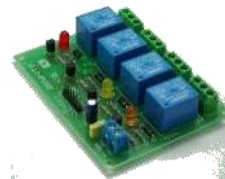
Fig .6 Relay Board
