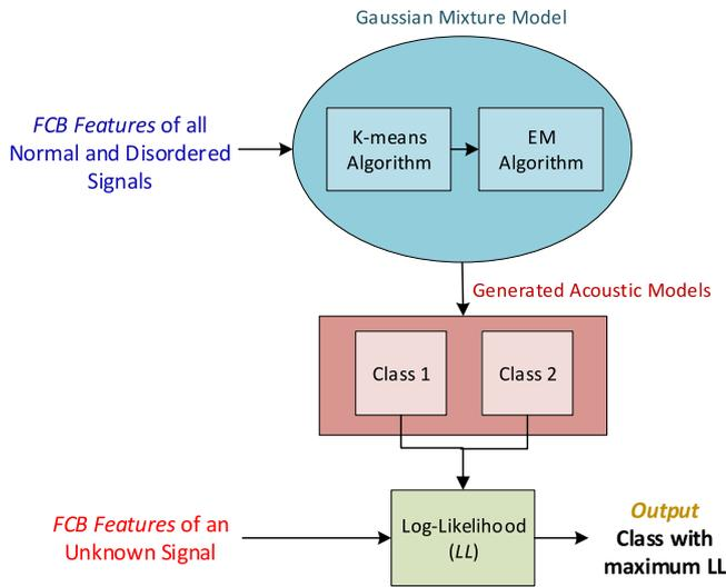
Fig. 5. Block diagram for the proposed detection and classification system.
