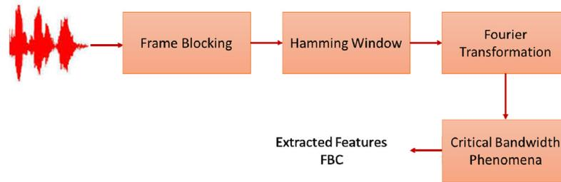
Fig. 3. The steps of acoustic analysis for extraction of the feature FCB.
