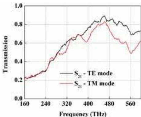
Figure 8. Measured transmission coefficient,  $S_{21}$ .
