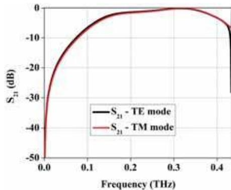
**Figure 5.** Transmission coefficient,  $S_{21}$  for TE and TM modes.
