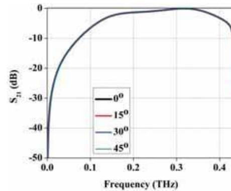
**Figure 6.** Transmission coefficient,  $S_{21}$  for different incident angles.
