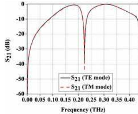
**Figure 2.**  $S_{21}$  of the FSS two-concentric hexagonal slot FSS structure.
