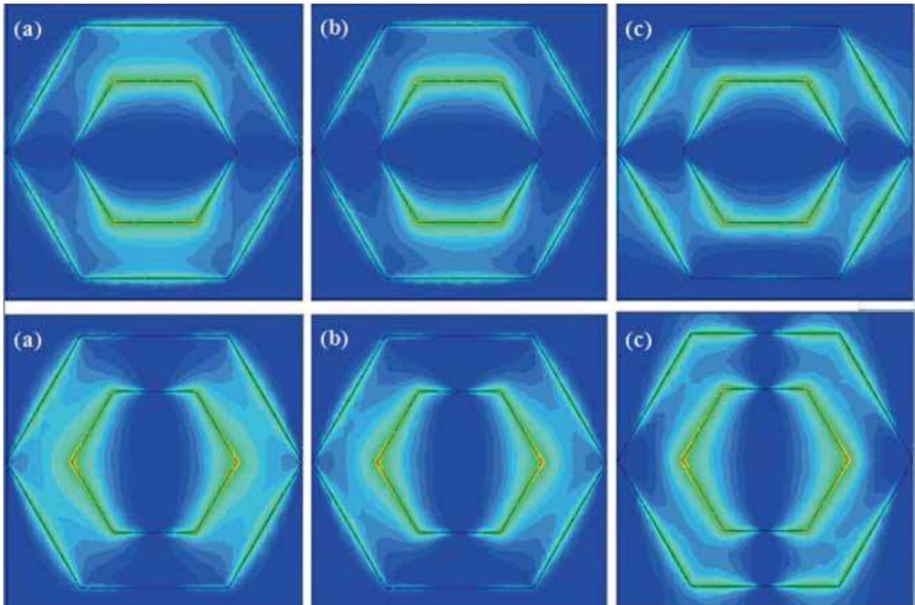
**Figure 10.** TE mode and TM mode electric field distribution at the three frequencies: (a) 0.2 THz, (b) 0.36 THz and (c) 0.52 THz.
