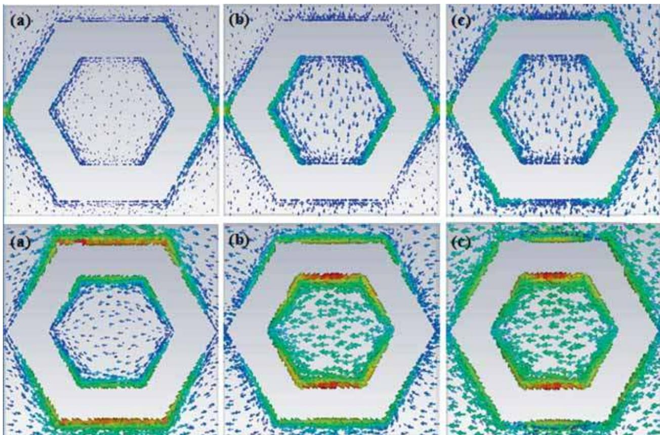
Figure 9. TE mode and TM mode surface current distribution at the three frequencies: (a) 0.2 THz, (b) 0.36 THz and (c) 0.52 THz.
