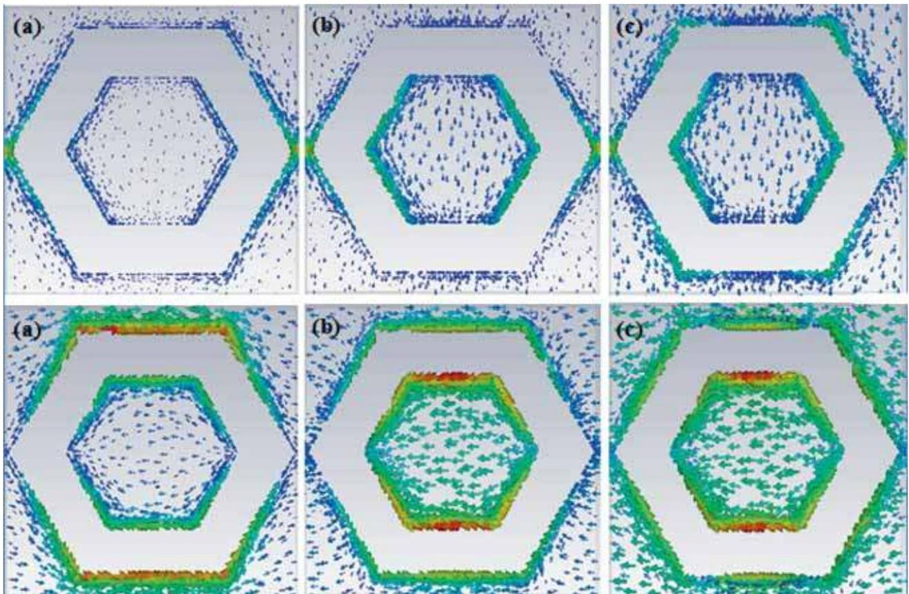
**Figure 9.** TE mode and TM mode surface current distribution at the three frequencies: (a) 0.2 THz, (b) 0.36 THz and (c) 0.52 THz.
