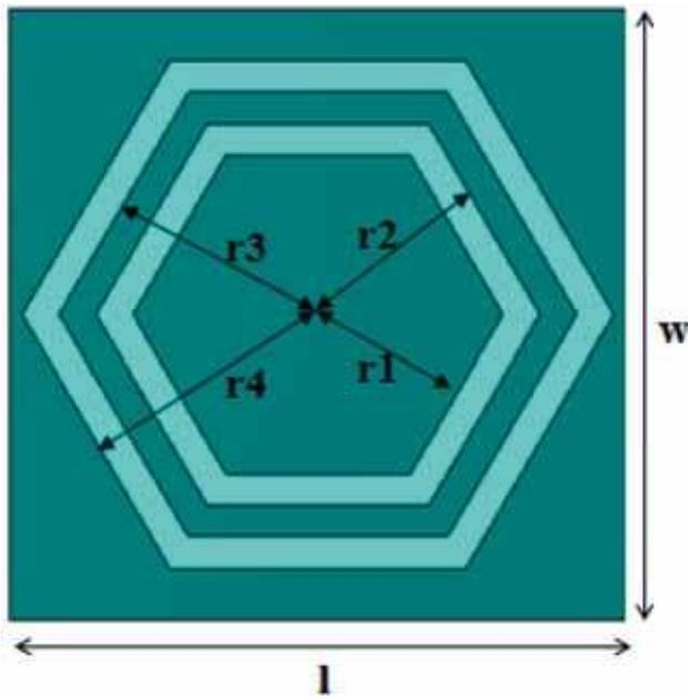
**Figure 1.** Schematic of the two-concentric hexagonal slot FSS filter structure.
