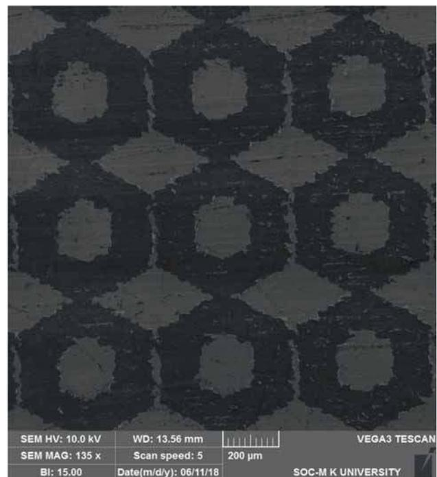
**Figure 7.** SEM image of the fabricated FSS filter.
