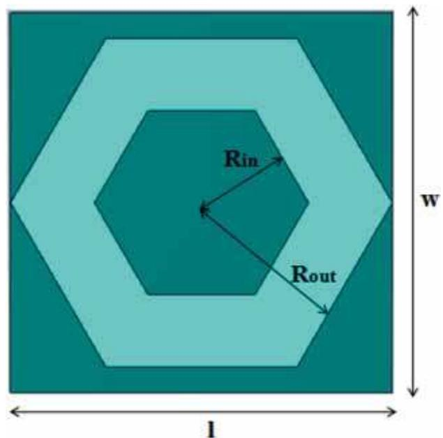
**Figure 3.** Schematic of the broadband FSS filter structure.
