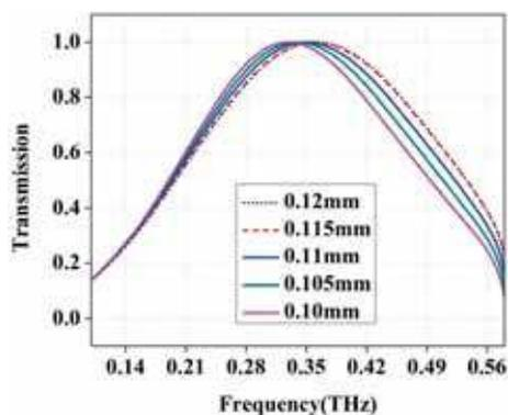
**Figure 11.** Transmission in dB for different widths of the hexagonal slot.
