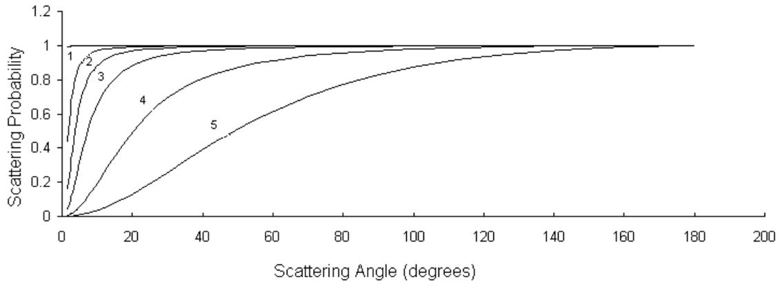
**Fig. 2.** Variation of the scattering probability with the angle of scattering in GaN at 77 K for different values of ionized impurity concentration. The average electron energy is 0.01 eV for all the curves. (1)  $1 \times 10^{13} \text{ cm}^{-3}$ , (2)  $5 \times 10^{13} \text{ cm}^{-3}$ , (3)  $1 \times 10^{14} \text{ cm}^{-3}$ , (4)  $5 \times 10^{14} \text{ cm}^{-3}$ , (5)  $1 \times 10^{15} \text{ cm}^{-3}$ , and (6)  $5 \times 10^{15} \text{ cm}^{-3}$ .
