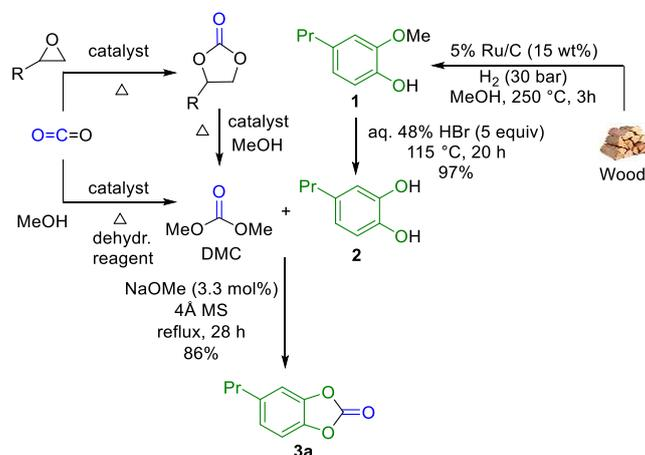
**Scheme 2.** Synthesis of 4-propylcatechol carbonate (**3a**) from 4-propylcatechol (**2**) and DMC obtained from wood and CO<sub>2</sub>, respectively.
