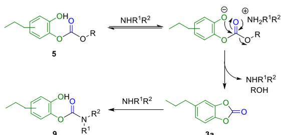
**Scheme 9.** Mechanism of formation of **9** from **5** and NHR<sup>1</sup>R<sup>2</sup>.
