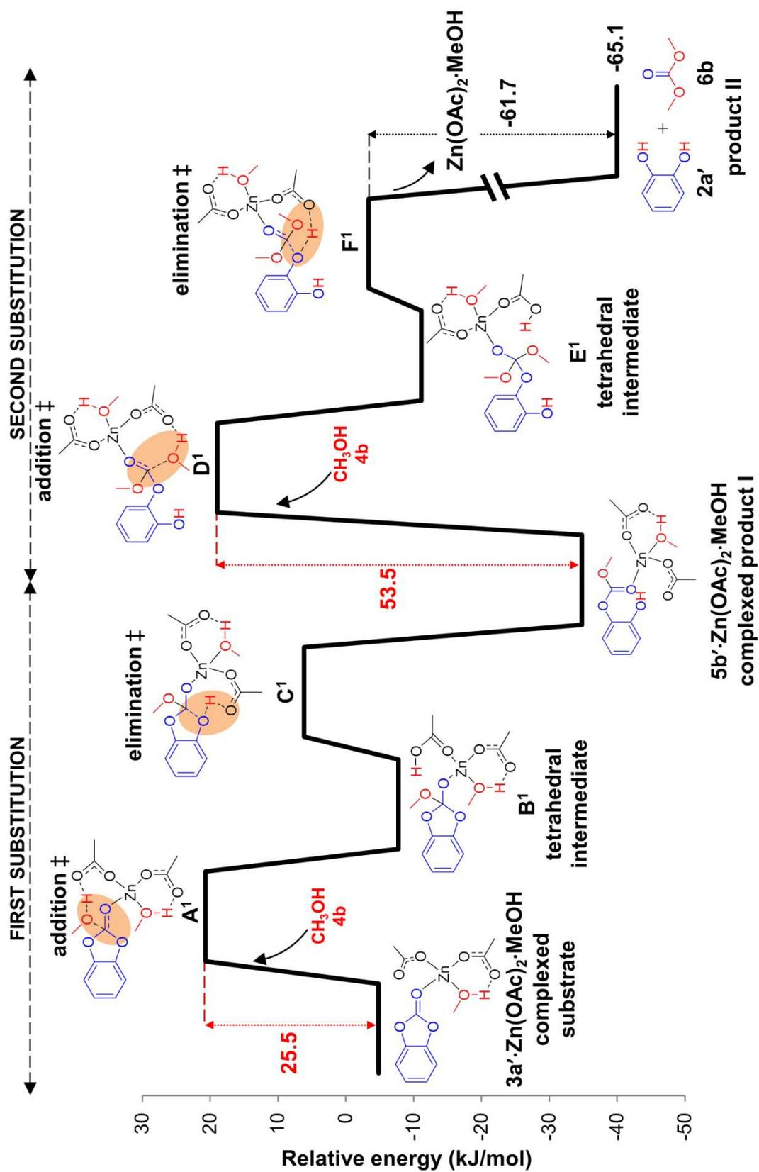
Figure 1. DFT calculation (B3LYP/6-31+G(d)) for the reaction of catechol carbonate (**3a'**) with methanol (**4b**) catalyzed by Zn(OAc)<sub>2</sub>·2H<sub>2</sub>O.
