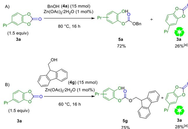
**Scheme 5.** Synthesis of A) benzyl 2-hydroxy-propylphenyl carbonates (**5a**) and B) (9H-fluoren-9-yl)methyl 2-hydroxy-propylphenyl carbonates (**5g**) at 15 mmol scale. [a] The recovered **3a** yield was calculated based on the initial amount of **3a** added (22.5 mmol). Considering full conversion of **4**, the recovered amount of **3a** has a maximum of 33%.
