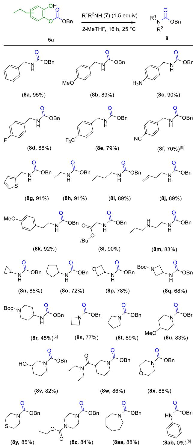
**Scheme 7.** Reaction of benzyl 2-hydroxy-propylphenyl carbonates (**5a**) with amines (**7**).<sup>[a]</sup> [a] Conditions: **5a** (1 mmol), **7** (1.5 mmol), rt, 16 h, 2-MeTHF (1 mL). Isolated yield. [b] 40 °C. [c] 45% of **9r** isolated.
