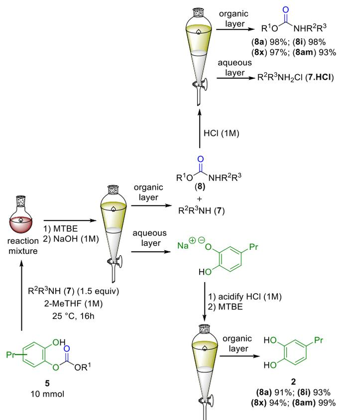
**Scheme 6.** Work-up of the synthesis of carbamates (**8**) at 10 mmol scale.
