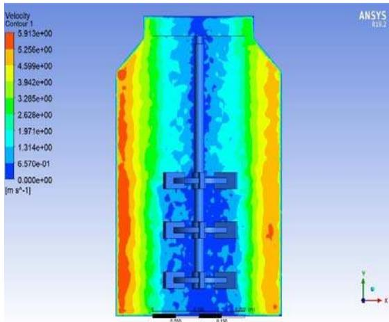
Figure 8. Velocity contour of multiple impeller
