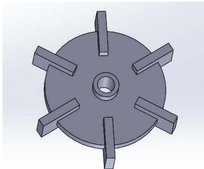
**Figure 1** Schematic diagram of impeller
