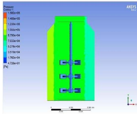
Figure 9. Pressure contour of multiple impeller
