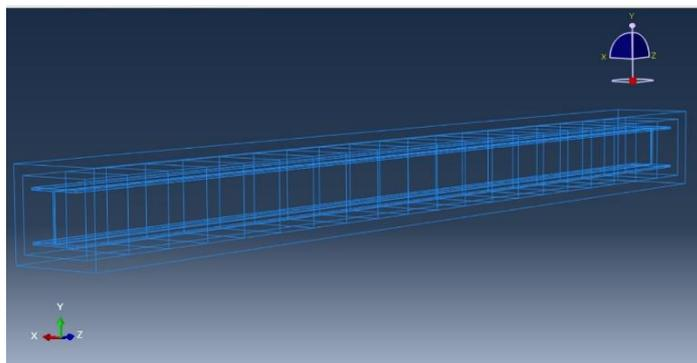
**Figure 9 -** Composite Column Model.
