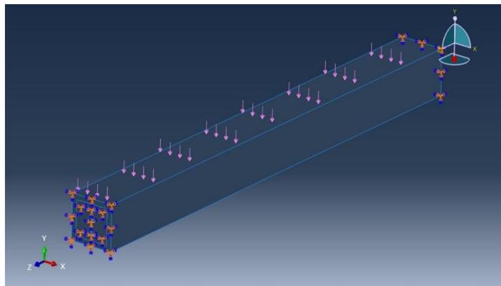
**Figure 12** - Loading of Composite Column.
