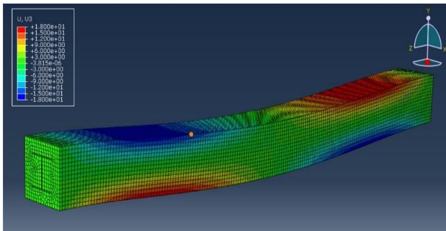
Figure 22 - Displacement (mm) along Z direction.
