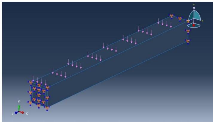
**Figure 12** - Loading of Composite Column.
