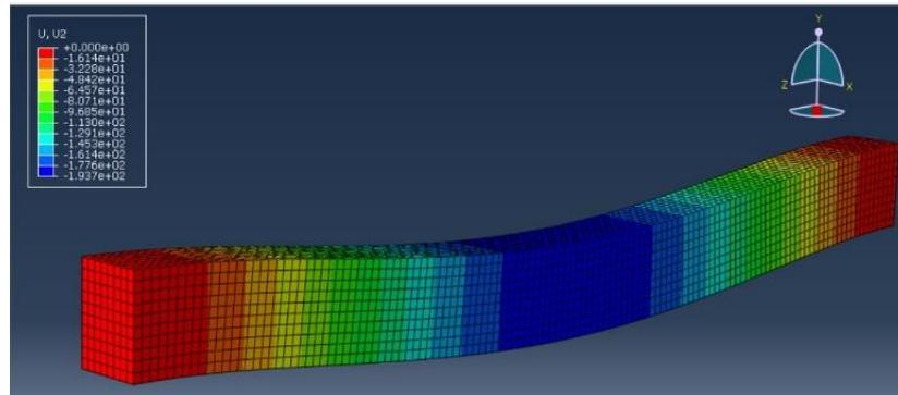
**Figure 16** - Displacement (mm) along Y direction.
