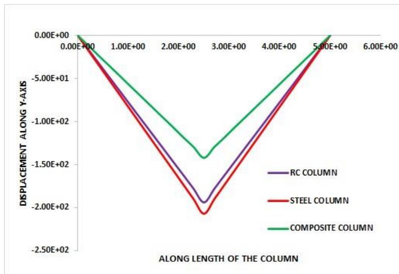
Figure 27 - Comparison of Displacement along C/S with RC column, Steel Column & Composite Column.
