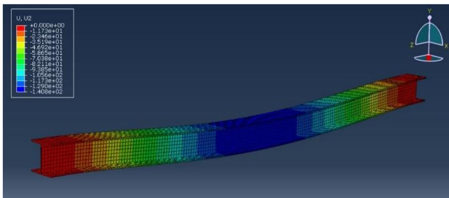
**Figure 25** - Displacement (mm) of steel in composite column along Y direction.
