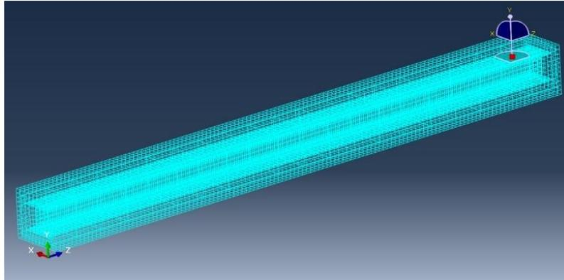
**Figure 11** - Meshing of Composite Column.
