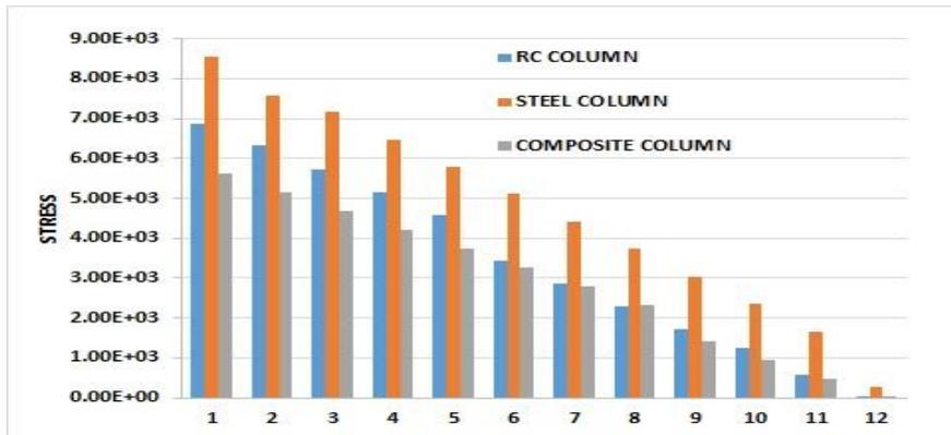
Figure 26 - Comparison of Stresses (MPa) with RC column, Steel Column & Composite Column.
