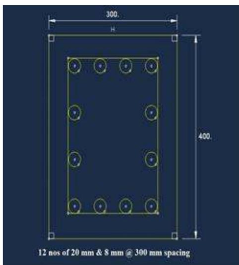
**Figure 1** - C/S Details of RC Column.
