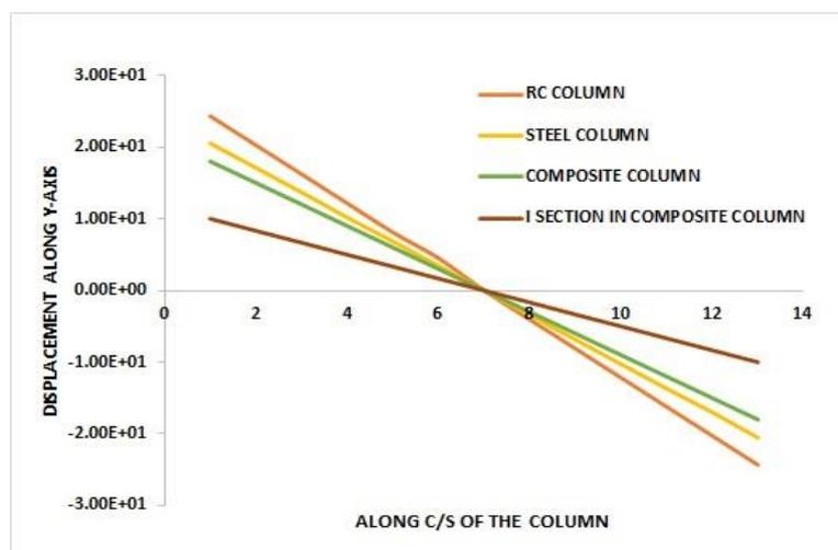
Figure 28 - Comparison of Displacement along Length with RC column, Steel Column & Composite Column.
