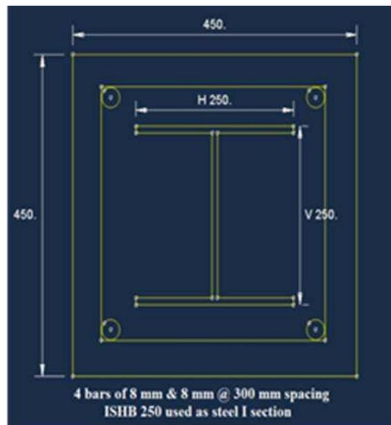
**Figure 3** - C/S Details of Composite Column.
