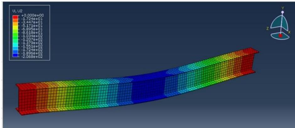
**Figure 19** - Displacement (mm) along Y direction.
