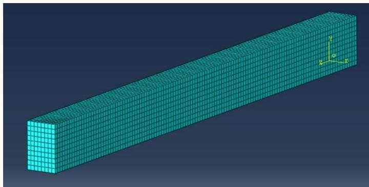
Figure 5 - Meshing of RC Column.
