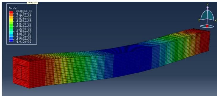
**Figure 24** - Displacement (mm) along Y direction.
