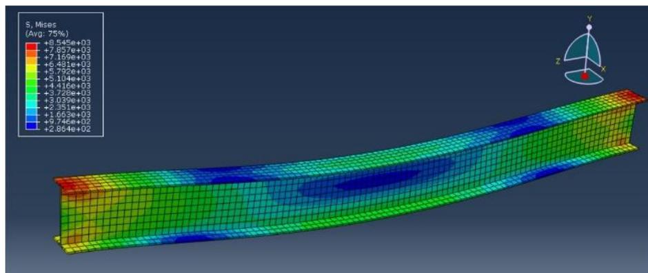
**Figure 17** - Stress (MPa) Distribution in steel column.
