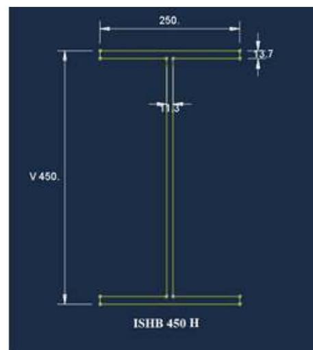
**Figure 2** - C/S Details of Steel Column ISHB 450.
