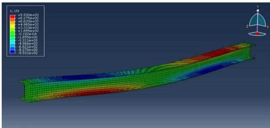
Figure 23 - Displacement (mm) of steel in composite column.
