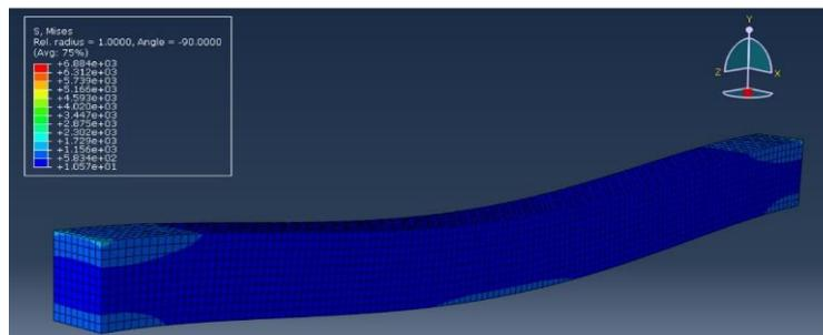
**Figure 14** - Stress (MPa) Distribution in RC Column.
