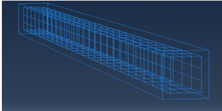
Figure 4 - Model of RC Column with Reinforcement.
