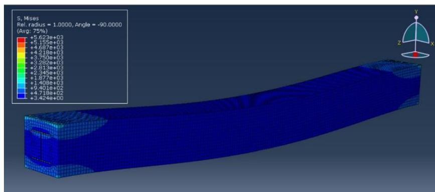
**Figure 20** - Stress (MPa) Distribution in composite column.
