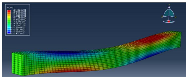
**Figure 15** - Displacement (mm) along Z direction.
