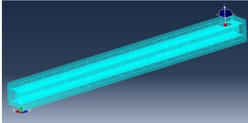
**Figure 11** - Meshing of Composite Column.
