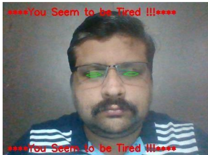
Figure 9. Person classified as feeling fatigue while wearing glasses and automated alert generated
