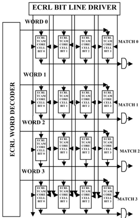
Fig. 7 TCAM array with the proposed ECRL (adiabatic) TCAM core cells and ECRL (adiabatic) peripheral circuits
