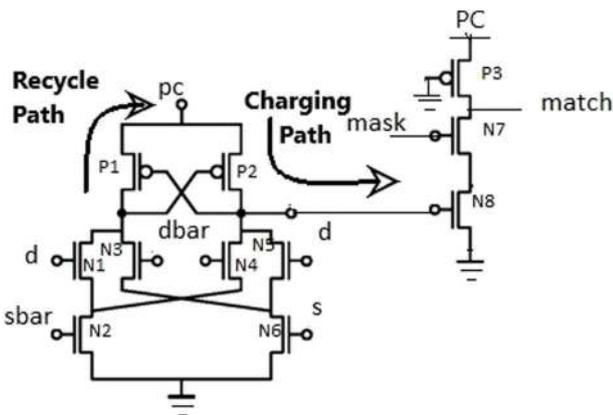
Fig. 3 Schematic diagram of the QATCAM cell based on ECRL
