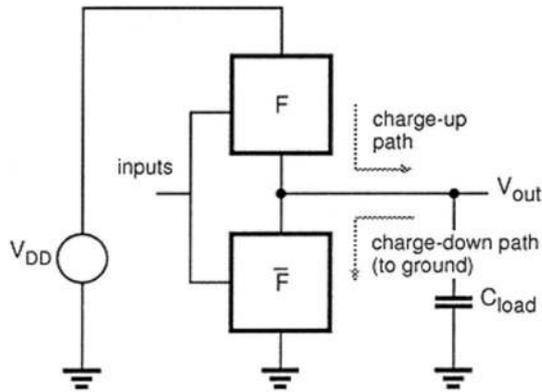
Fig. 1 Conventional CMOS structure [29]
