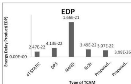
**Fig. 14** Comparison of EDP of the proposed TCAM along with its conventional counterparts
