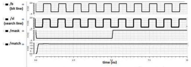
Fig. 8 Match output of the QATCAM cell based on ECRL
