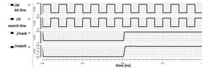
Fig. 11 Mismatch output of the QATCAM cell based on modified ECRL
