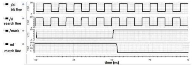
Fig. 9 Mismatch output of the QATCAM cell based on ECRL
