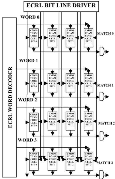
Fig. 6 TCAM array with conventional TCAM core cells and ECRL (adiabatic) peripheral circuits
