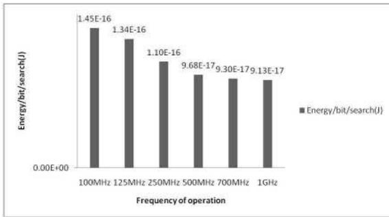
Fig. 15 Performance analysis of QATCAM cell based on MECRL at different frequencies
