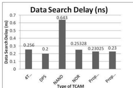
**Fig. 13** Comparison of data search delay of the proposed TCAM along with its conventional counterparts
