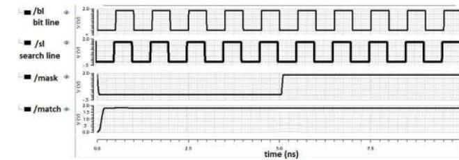
Fig. 10 Match output of the QATCAM cell based on modified ECRL
