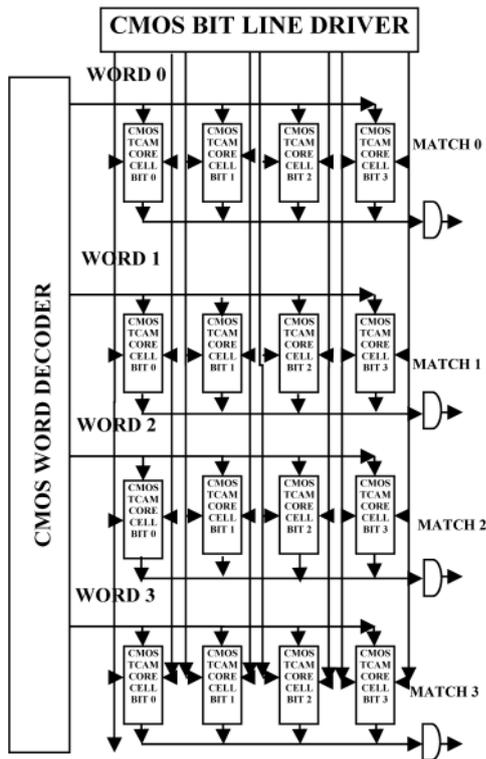
**Fig. 5** TCAM array with conventional TCAM core cells and CMOS peripheral circuits
