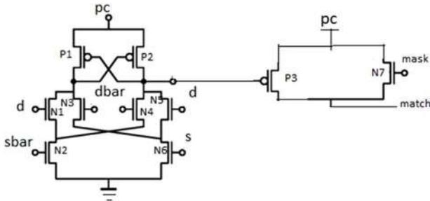
**Fig. 4** Schematic diagram of the QATCAM cell using modified ECRL
