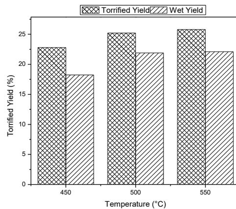
**Figure 5.** Pyro-oil yield for torrified and wet biomass
