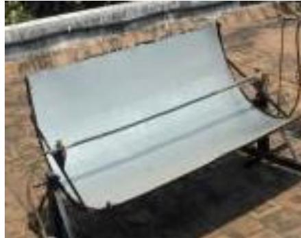
**Figure 4.** Parabolic solar collector
