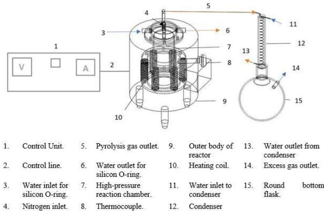
**Figure 2.** Fixed bed pyrolysis reactor for Sugarcane waste
