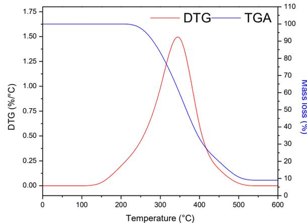
**Figure 3.** DSC/TGA analysis of sugarcane waste
