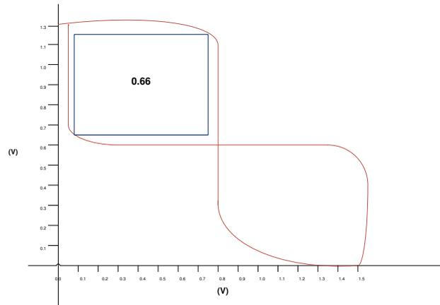
**Figure 5.** Static Noise Margin (SNM) of 8T SRAM cell.
