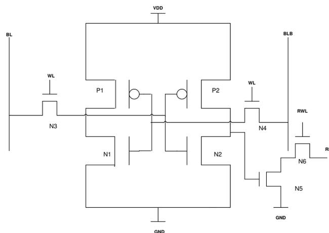
**Figure 1.** Conventional 8T SRAM cell
