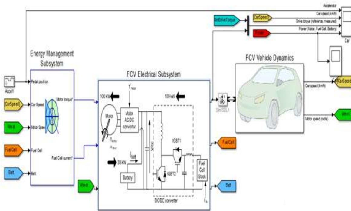
**Figure 3.** Proposed system of the 100-kW fuel cell vehicle.
