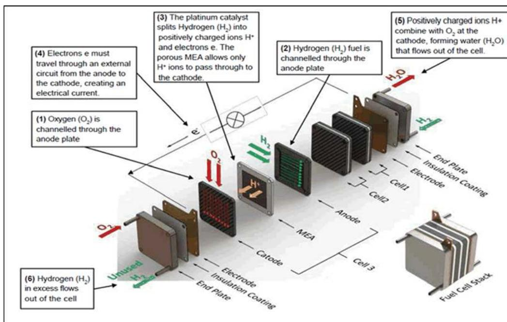
**Figure 1.** Layout and operation of PEMFC.
