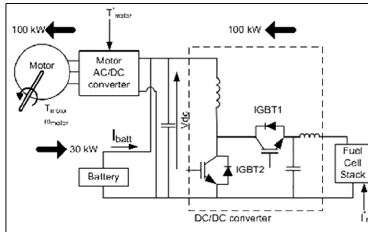
**Figure 4.** FCV electrical subsystem.
