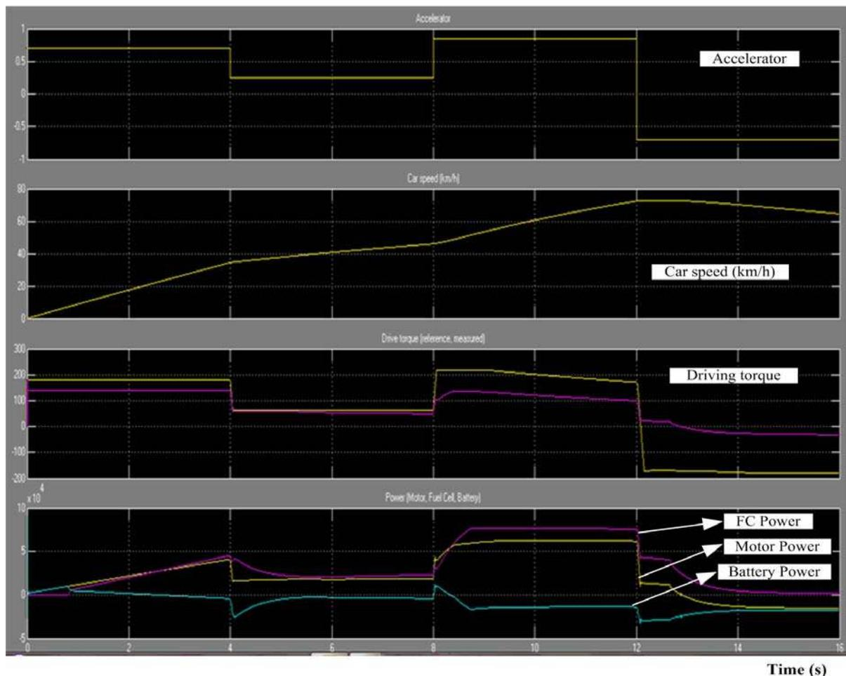
**Figure 5.** Simulation results and power outputs throughout the full driving cycle.
