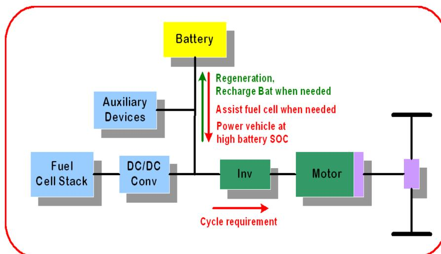
**Figure 2.** Fuel cell power conversion system components.
