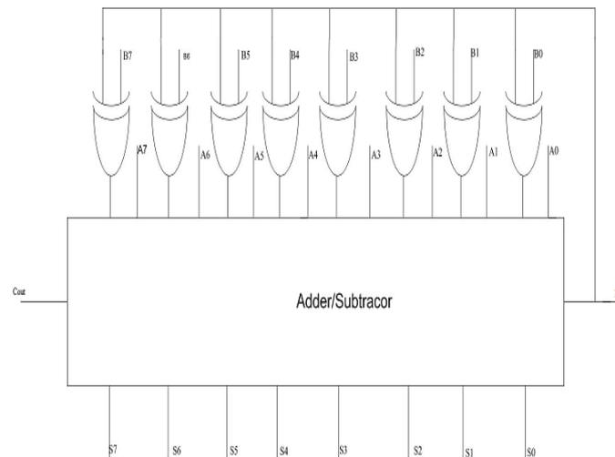
**Figure 3.** Adder – Subtractor unit
