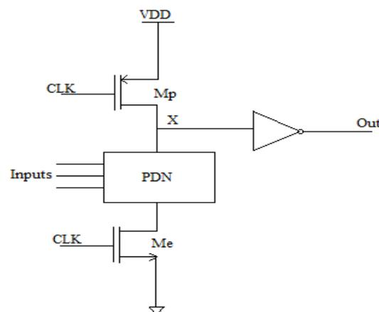
**Figure 1.** Conventional Domino logic circuit
