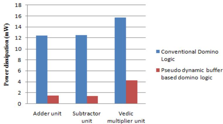
**Figure 6.** Power comparison of 8bit arithmetic unit of ALU
