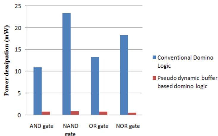
**Figure 7.** Power comparison of 8 bit logical unit of ALU
