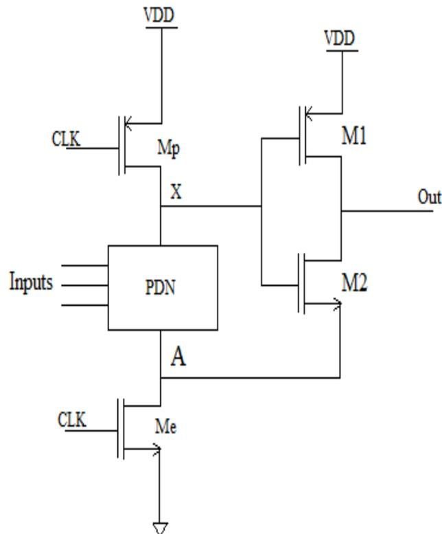
**Figure 2.** PDB based domino logic circuit
