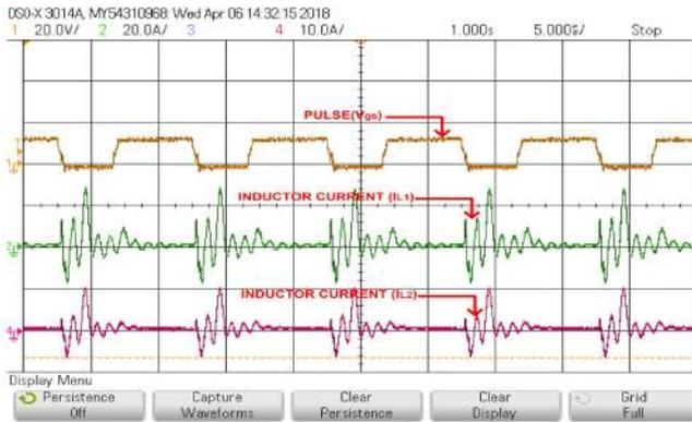
Fig. 8 Inductor currents of  $L_1$  and  $L_2$
