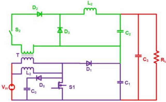
**Fig. 3** Proposed hybrid converter circuit
