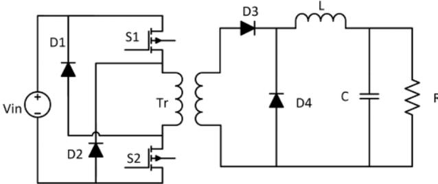
Fig. 2 Circuit diagram of a forward converter
