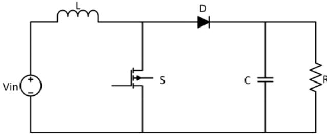
Fig. 1 Circuit diagram of a boost converter
