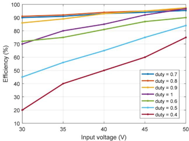
Fig. 11 Performance of hybrid converter
