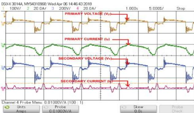
Fig. 9 Transformer waveforms: brown-primary voltage; green-primary current; blue-secondary voltage; pink-secondary current
