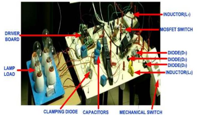
Fig. 7 Proposed hybrid converter
