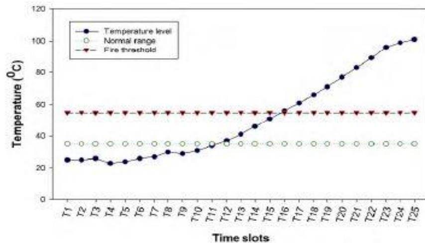
**Figure 11.** Result of fire level monitoring system of existing system. Courtesy (“Towards Disaster Resilient Smart Cities: Can Internet of Things and Big Data Analytics Be the Game Changers?”, IEEE trans. on special section on urban computing and intelligence.)
