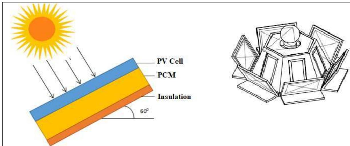
**Fig 1.** (a) Schematic of passive cooling system with PCM (b) CAD model of the new P-V module
