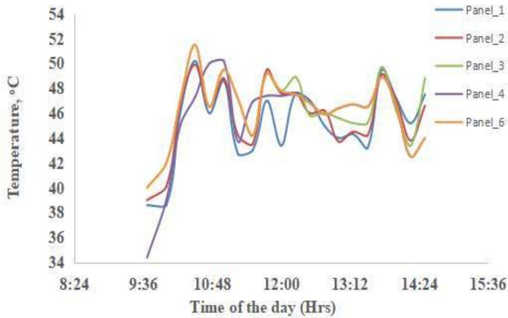
Fig 5. Influence of different time of the day on the changes in panel surface temperature
