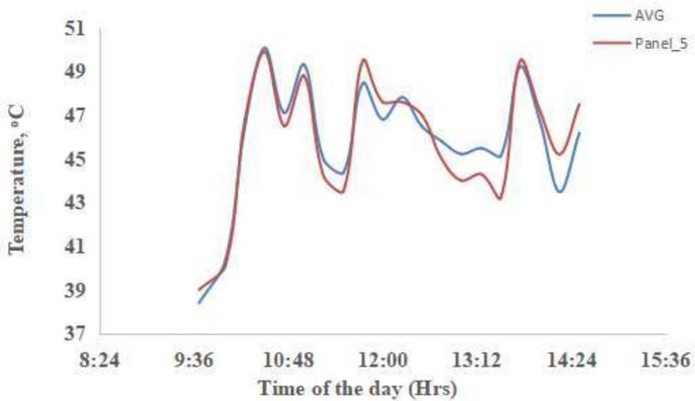
Fig 6. Average value of temperature curves in comparison with the PCM reinforced panel
