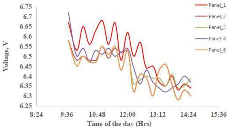
**Fig 3.** Influence of different time of the day on the changes in panel voltage
