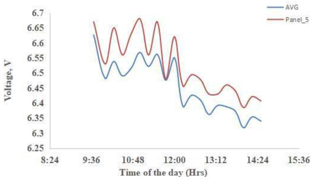
**Fig 4.** Average value of voltage curves in comparison with the PCM reinforced panel
