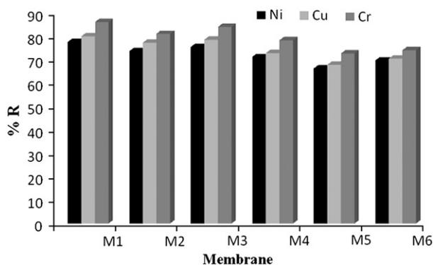
Fig. 4. Solvents effect and solvents composition in PES membranes on rejection of Cu(II), Ni(II) and Cr(III) metal ions with PVA microligand.
