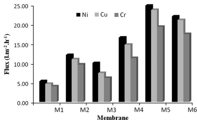
Fig. 6. Solvents effect and solvents composition in PES membranes on permeate rate (flux) of Cu(II), Ni(II) and Cr(III) metal ions with PVA microligand.
