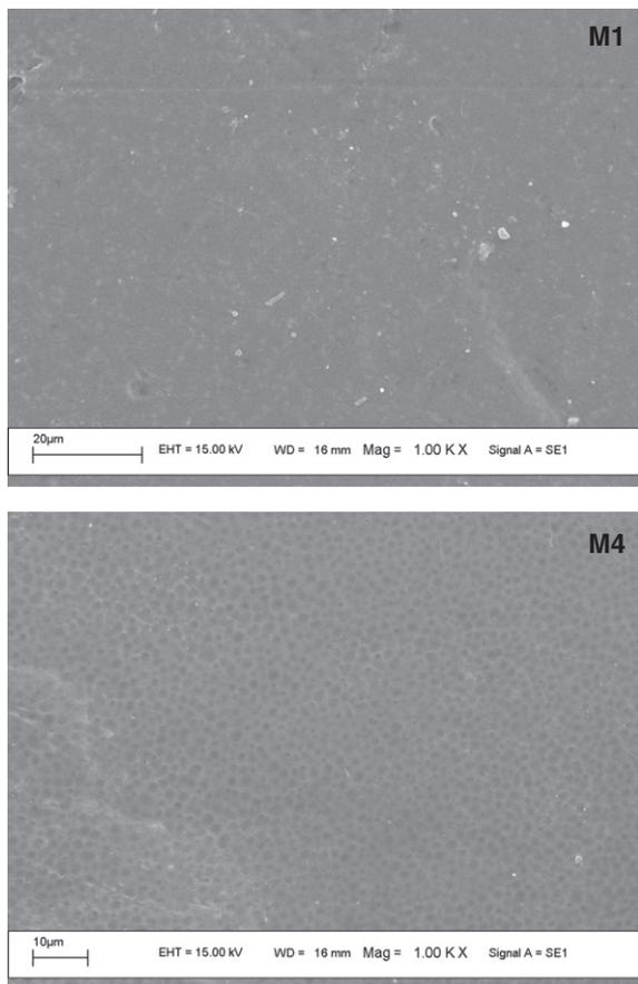
Fig. 1. SEM photographs of the top surface of membranes formed from 82.5 (M1) and 85% (M4) of NMP in 17.5 and 15% of PES respectively, magnification 1000.
