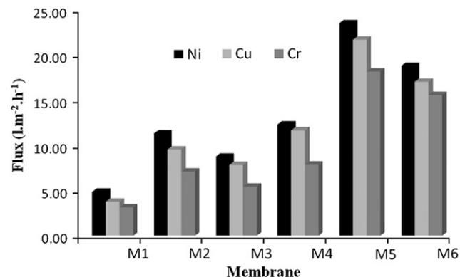
Fig. 7. Solvent effect and solvent composition in PES membranes on permeate rate (flux) of Cu(II), Ni(II) and Cr(III) metal ions with PDDA microligand.
