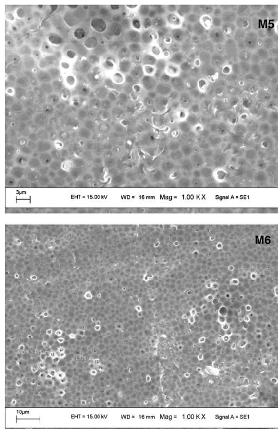
Fig. 2. SEM photographs of the top surface of membranes formed from 85% of DMSO (M5) and DMF (M6) as solvents in 15% PES polymer, magnification 1000.
