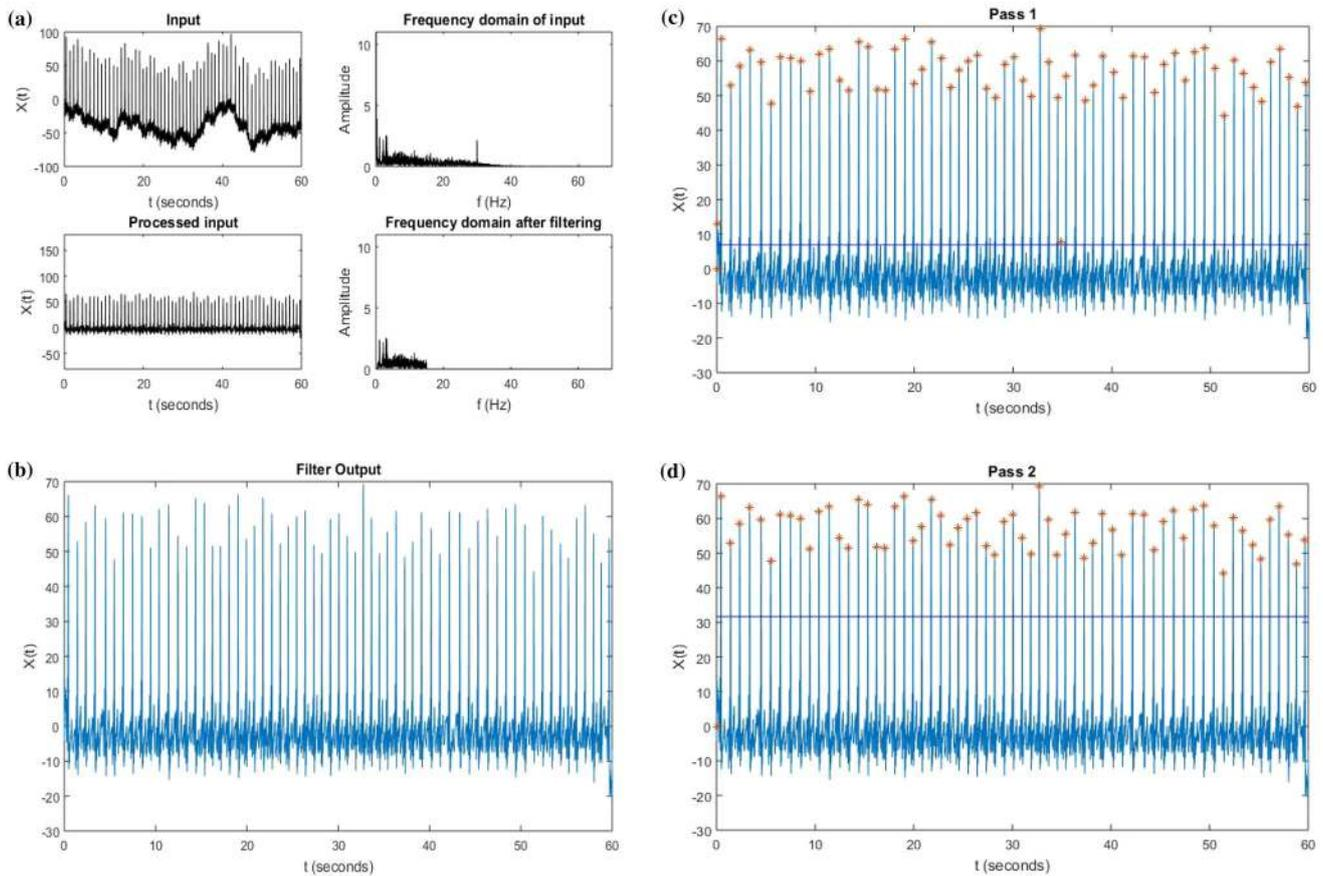
**Fig. 4** The output of the proposed algorithm. *Note:* The 115.mat input ECG signal taken from the MITADB is represented in **a**, with the denoising process shown using 4 subplots. **b** The output of the FFT based bandpass filter. **c** The result of the first pass in the R-peak
