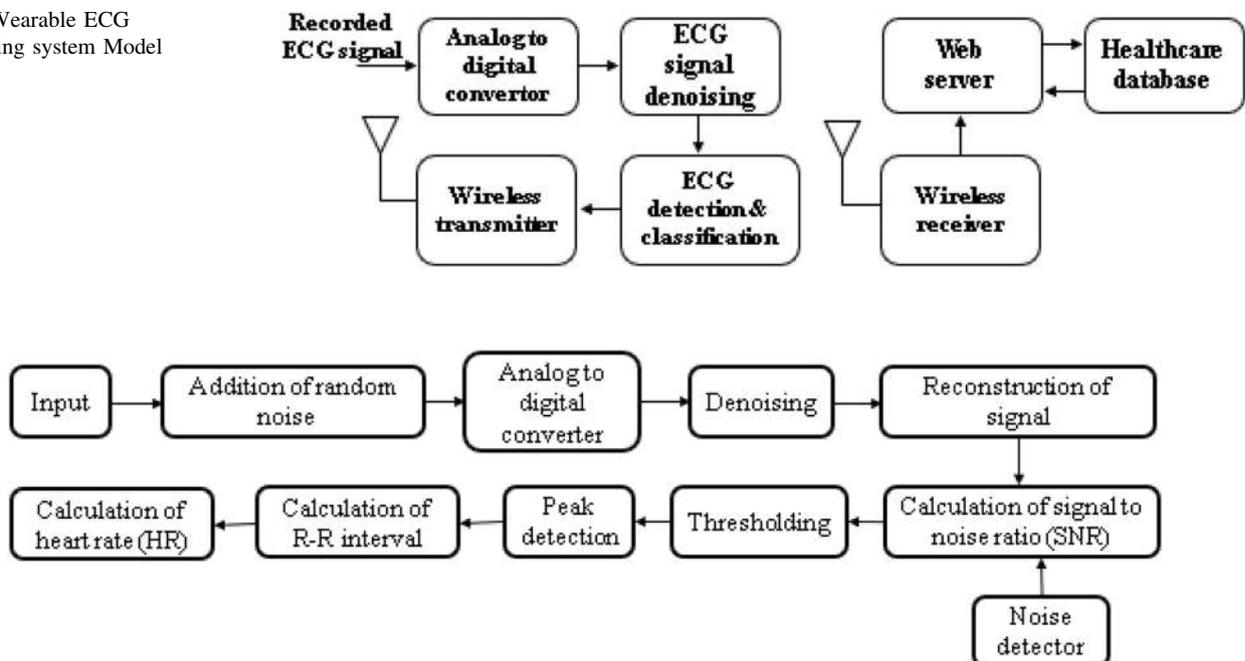
Fig. 3 Block diagram representation of the proposed FFT based ECG denoising and adaptive R-peak detection algorithm
