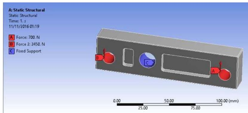
**Figure 6** FEM (deformation) of hydraulic calliper mount in ANSYS (see online version for colours)
