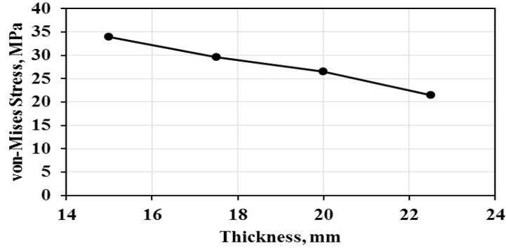
**Figure 13** Graph showing von Mises stress versus thickness of lever arm (Class 1)
