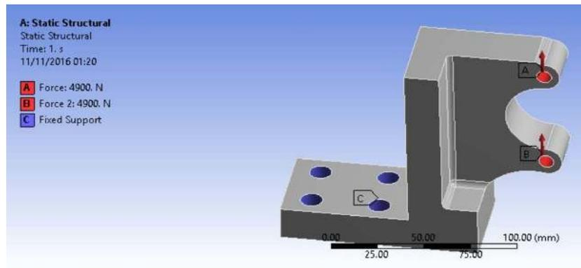
**Figure 5** Boundary conditions for lever arm (see online version for colours)
