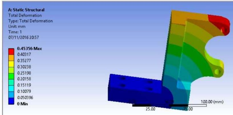
**Figure 7** FEM (von Mises stress) of hydraulic calliper mount in ANSYS (see online version for colours)
