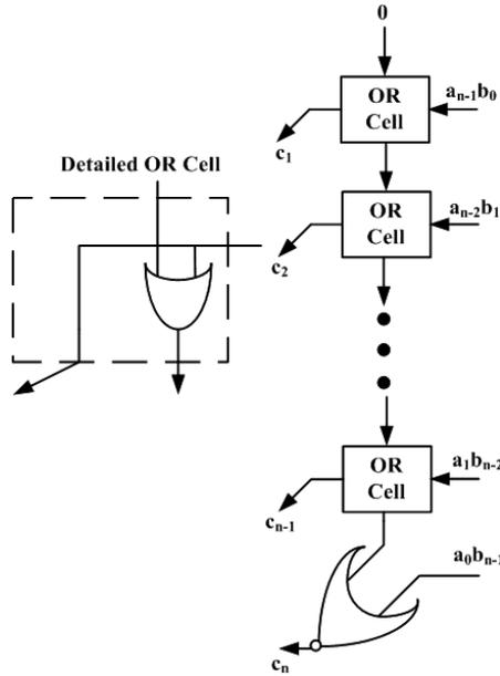
Fig. 8. Van 2005 correction logic for signed multiplier,  $w = n$  and  $h = 0$ .
