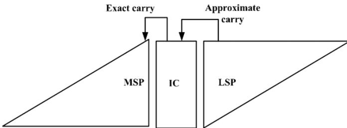
Fig. 4. General scheme of a fixed-width multiplier.
