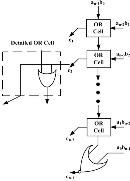
Fig. 6. Jou 99 correction logic for signed multiplier,  $w = n$  and  $h = 0$ .
