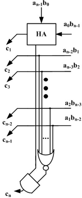
Fig. 10. Strollo Type I correction logic for unsigned multiplier,  $w = n$  and  $h = 0$ .
