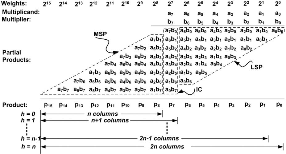
Fig. 1. Subdivision of the matrix of partial products, for unsigned multiplier,  $n = 8$  with  $h = 0$ .
