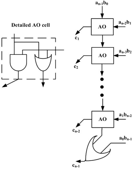
Fig. 9. Curticapean 2001 correction logic for unsigned multiplier,  $w = n$  and  $h = 0$ .
