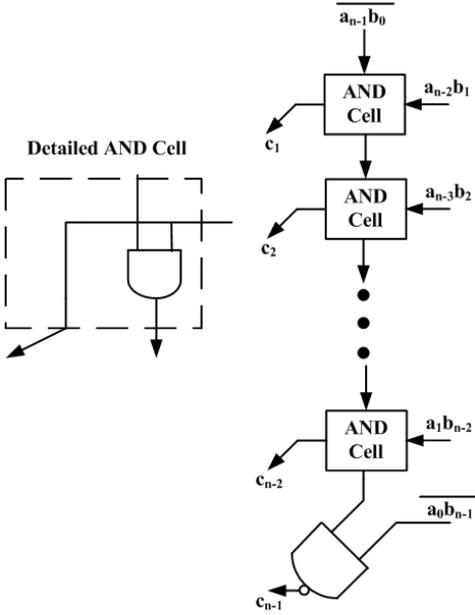
Fig. 7. Van 2000 correction logic for signed multiplier,  $w = n$  and  $h = 0$ .
