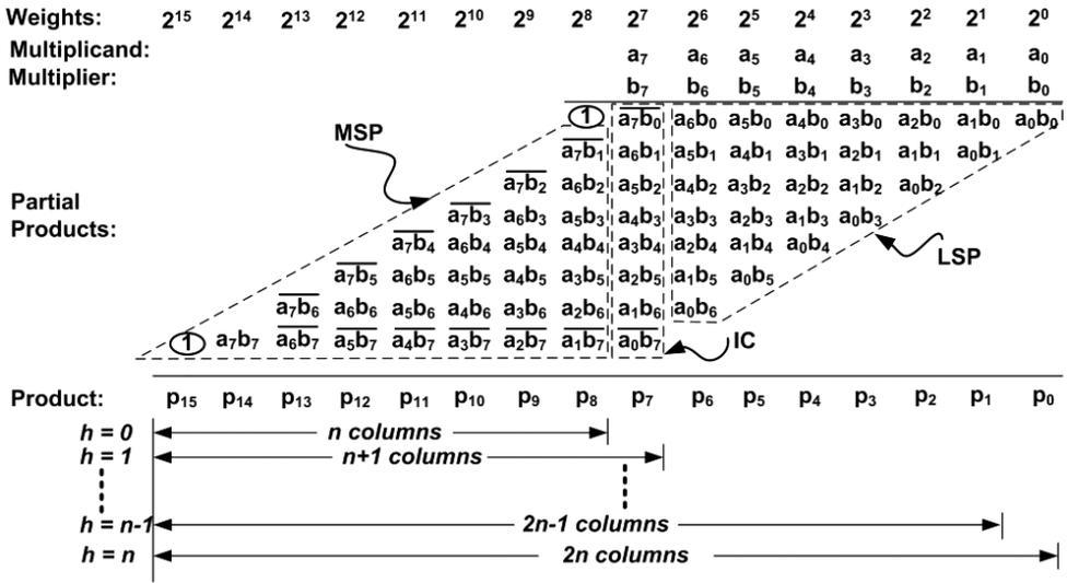
Fig. 2. Subdivision of the matrix of partial products, for Baugh-Wooley array multiplier,  $n = 8$  with  $h = 0$ .
