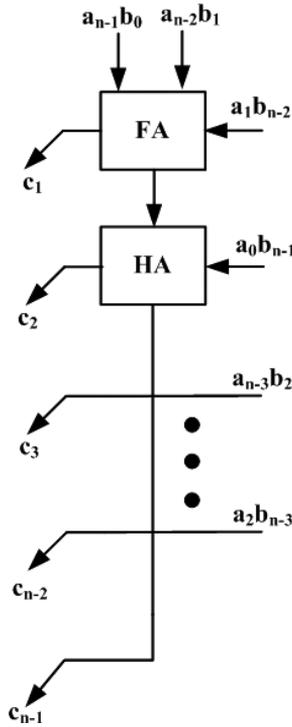
Fig. 11. Stollo Type II correction logic for unsigned multiplier,  $w = n$  and  $h = 0$ .
