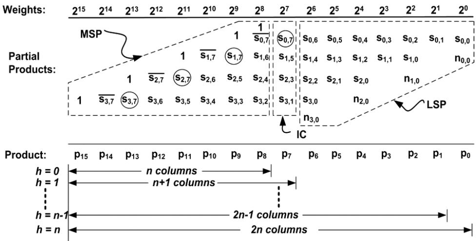
Fig. 3. Subdivision of the matrix of partial products, for modified Booth multiplier,  $n = 8$  with  $h = 0$ .
