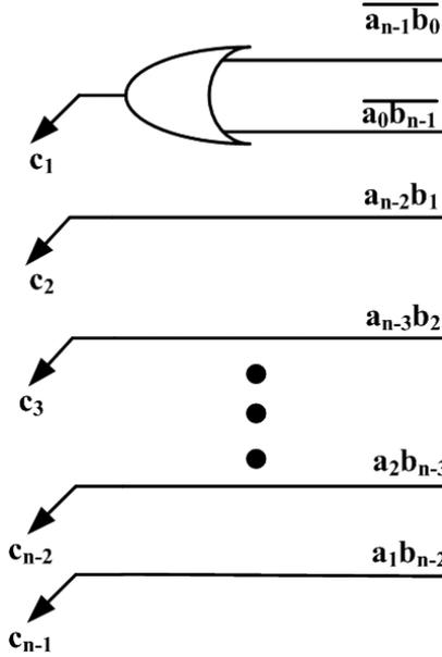
Fig. 14. Wang and Kuang correction logic for signed multiplier,  $w = n$  and  $h = 0$ .
