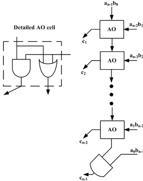
Fig. 5. Jou 99 correction logic for unsigned multiplier,  $w = n$  and  $h = 0$ .
