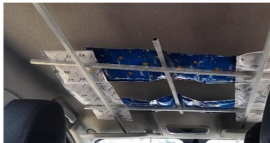
**Figure 2.** PCM at the Roof of the Car
