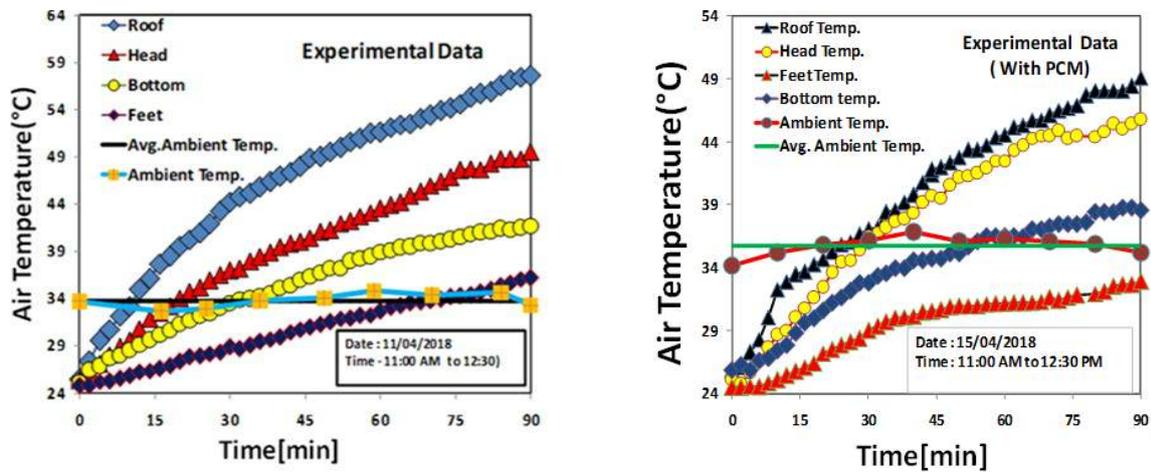
Figure 4. Air Temperature at different intervals of time (without PCM & With PCM).
