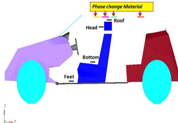
**Figure 3.** Positioning of Thermocouple at various locations.
