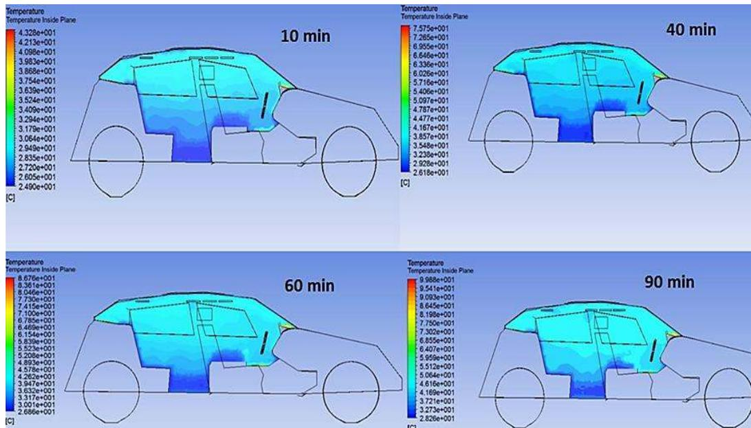
Figure 6 Contours of Air Temperature distribution along a plane at intervals of time
