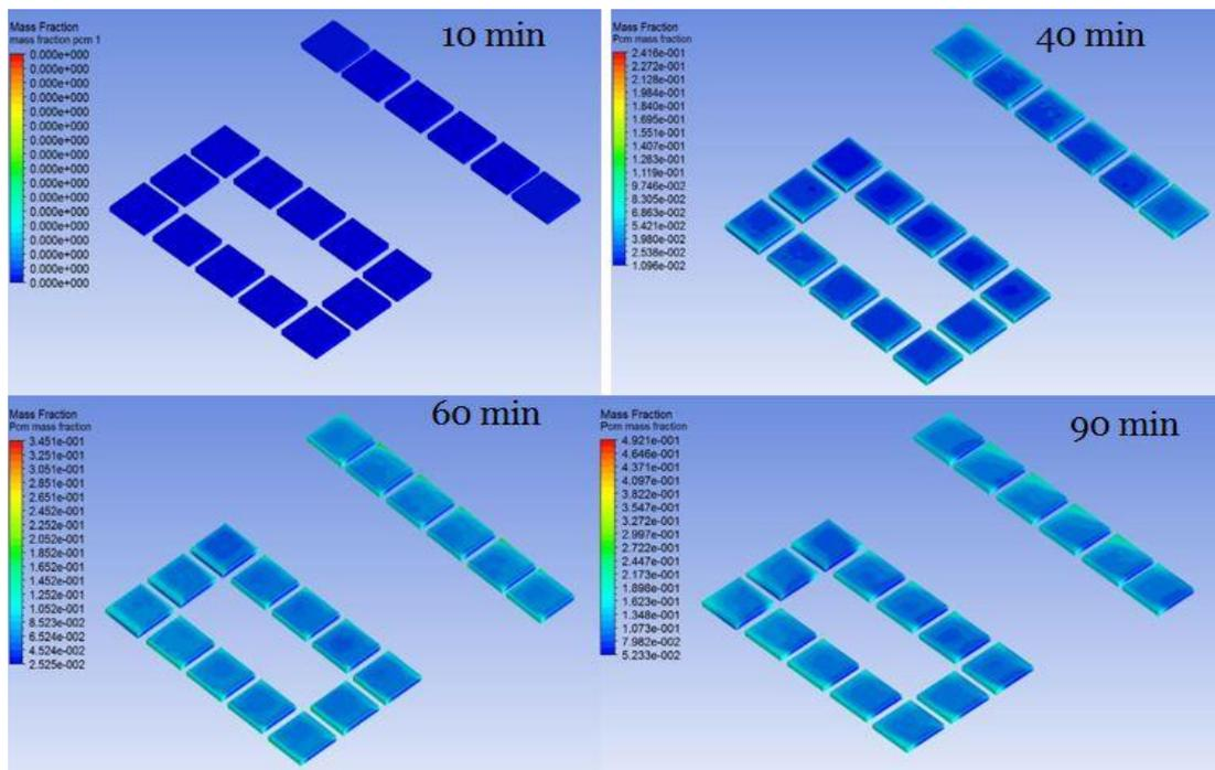
Figure 7 Liquid mass fraction of PCM
