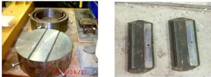
Figure-6. Loading caps for eccentric loads (Hadi, 2009)
