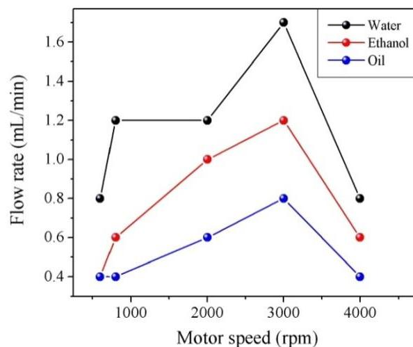
**Figure 5.** Flow rate of water, ethanol and coconut oil through the fabricated micropump Viscosities of water, ethanol and oil
