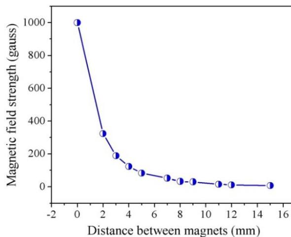
**Figure 2.** Magnetic field with a varying distance
