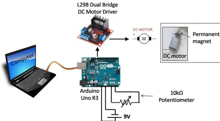
**Figure 3.** Schematic diagram showing the electrical circuit used to control DC motor speed
