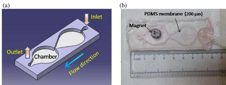
**Figure 1.** (a) CAD model of the dual chamber PDMS micropump with nozzle diffuser (b) Fabricated PDMS micropump with actuation magnet attached to its membrane
