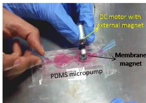
**Figure 4.** Photograph of flow rate measurement for water using fabricated PDMS micropump
