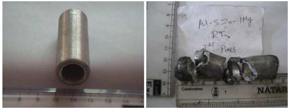
Fig. 5 Al-5Zn-1Mg tubular specimen before and after the first pass
