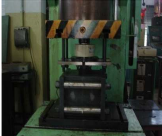
Fig. 3 Experimental setup of ECAP
