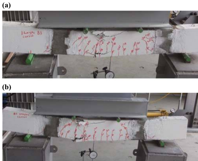
Notes: (a) Rupture of GFRP with the concrete crushing failure of beam FSB-CA1; (b) rupture of GFRP with the concrete crushing failure of beam FSB-CA2
