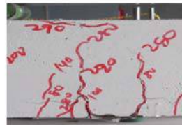
Plate 3. Failure pattern of the second series beams with one and two layers of bi-directional GFRP reinforcement
