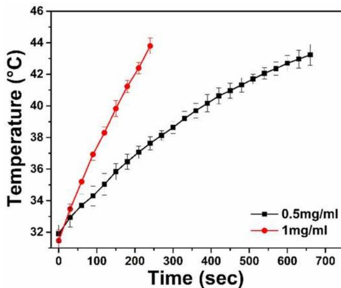
**Fig. 4** Temperature versus time graph of SPION with different concentration at frequency of 312 kHz and current of 235.2 A
