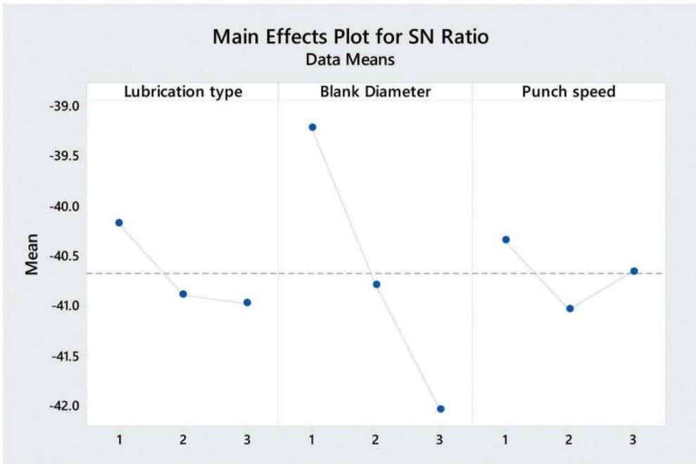
**Figure 5.** Effect of parameters on average S/N ratios.
