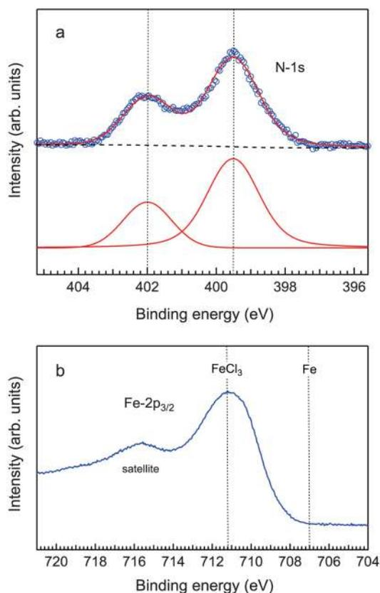
Fig. 4 XPS core level spectra acquired on  $\text{FeCl}_3$ -loaded hP2VP (loading ratio 0.3): N-1s binding energy range revealing 2 components (a) and Fe-2p<sub>3/2</sub> core level region giving evidence for the conservation of the oxidation state of the Fe after metal–organic complex formation (b).
