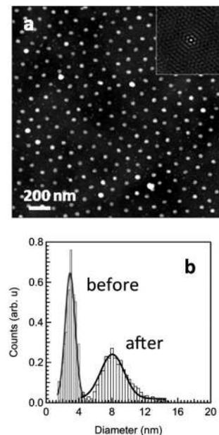
Fig. 5 AFM image (a) and related size distribution (b) of nanoparticles produced by adding additional  $\text{NbCl}_5$  to a micellar solution which has been pre-loaded by salt-decorated hP2VP (loading ratio 0.18). Clearly, the size of the resulting particles is increased without a significant loss of hexagonal order.
