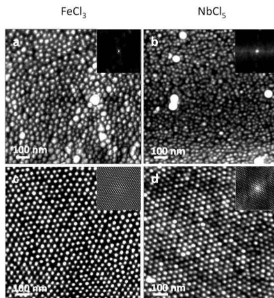
Fig. 1 AFM images demonstrating the poor lateral order of micellar monolayers on Si substrates loaded *directly* into solution with FeCl<sub>3</sub> (a) and NbCl<sub>5</sub> (b) metal precursors ('conventional' technique). Using our new approach, a significantly improved lateral order can be achieved for both FeCl<sub>3</sub> (c) as well as NbCl<sub>5</sub> (d) loaded micelles. The insets represent the auto-covariance functions of the corresponding AFM images.
