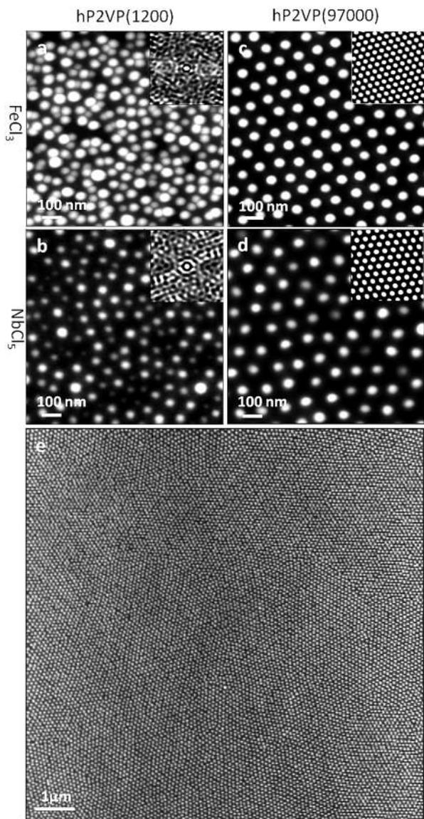
Fig. 2 AFM images and related auto-covariance functions (insets) of micellar patterns obtained from PS(185 000)-*b*-P2VP(90 000) based solutions that are loaded by  $\text{FeCl}_3$  and  $\text{NbCl}_5$ , using hP2VP(1200) (a and b) and hP2VP(97 000) (c and d) as precursor carriers; (e) represents a larger scan range of the sample shown in (c).
