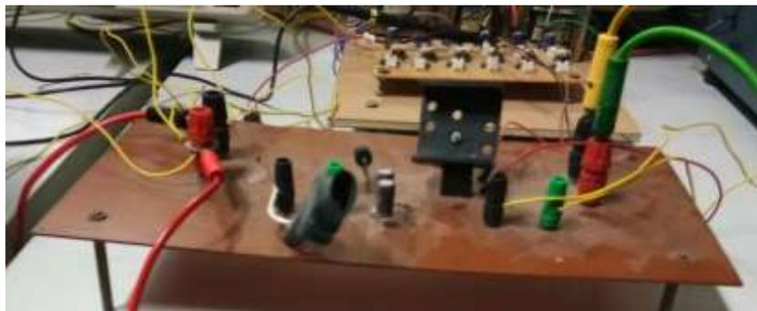
**Figure 5.** Hardware model of Cuk converter
