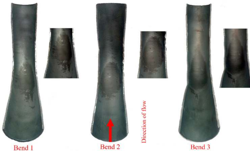
Fig. 11. Worn surfaces of test bends.
