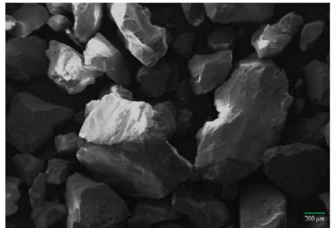
Fig. 3. SEM microphotographs of Fresh erodent material (Silica sand).
