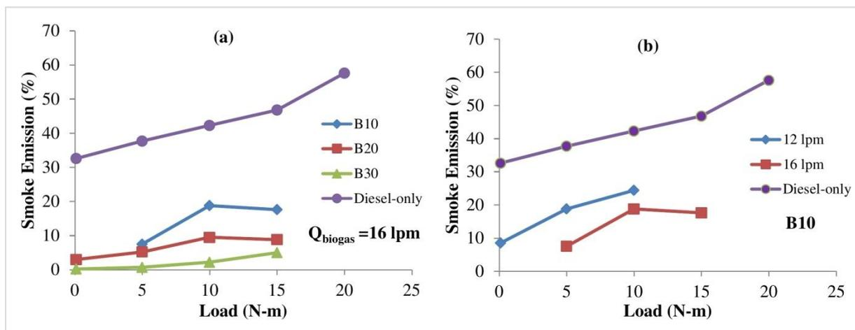
Figure 7: Effect of (a) butanol blending ratio and (b) biogas flow rate on smoke emission
