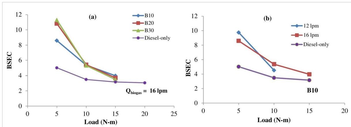
Figure 3: Effect of (a) butanol blending ratio and (b) biogas flow rate on BSEC
