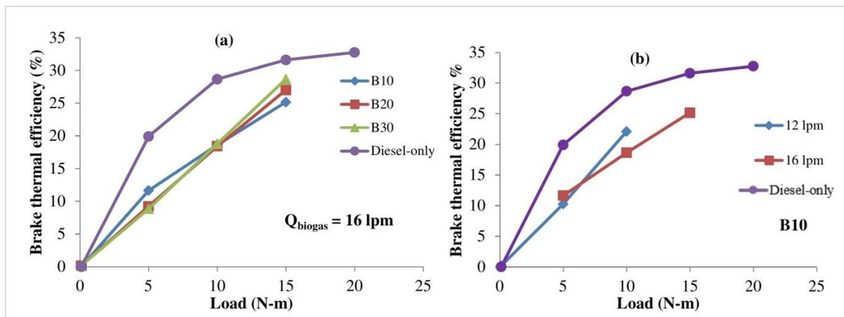
**Figure 2:** Effect of (a) butanol blending ratio and (b) biogas flow rate on brake thermal efficiency
