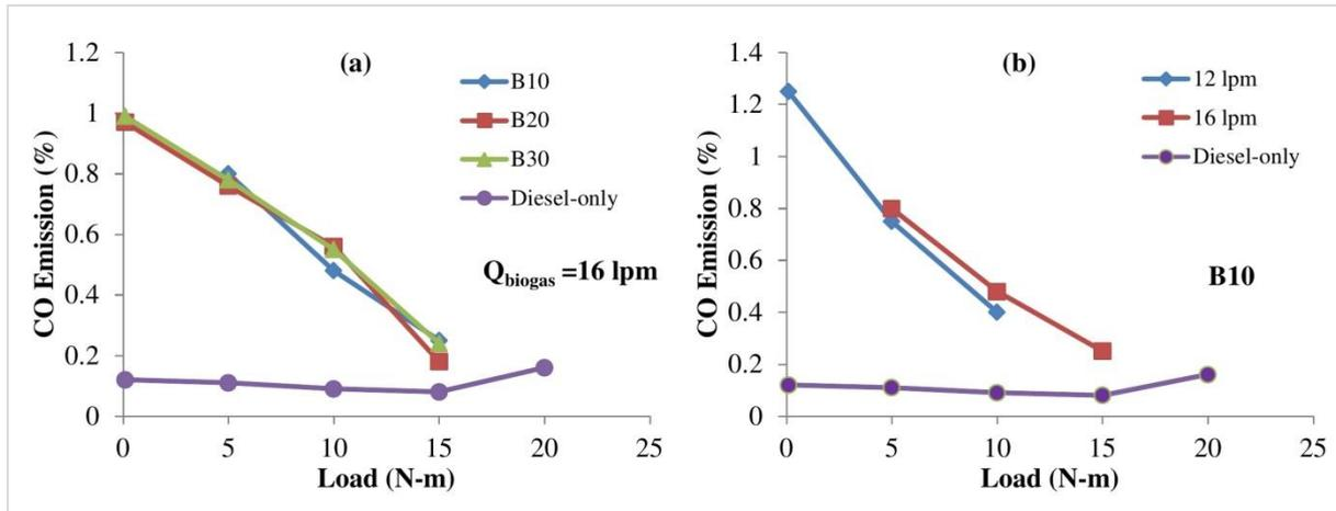
Figure 5: Effect of (a) butanol blending ratio and (b) biogas flow rate on CO emission
