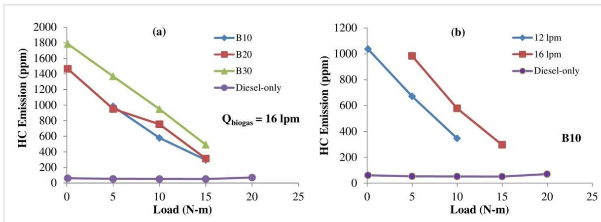
Figure 4: Effect of (a) butanol blending ratio and (b) biogas flow rate on HC emissions
