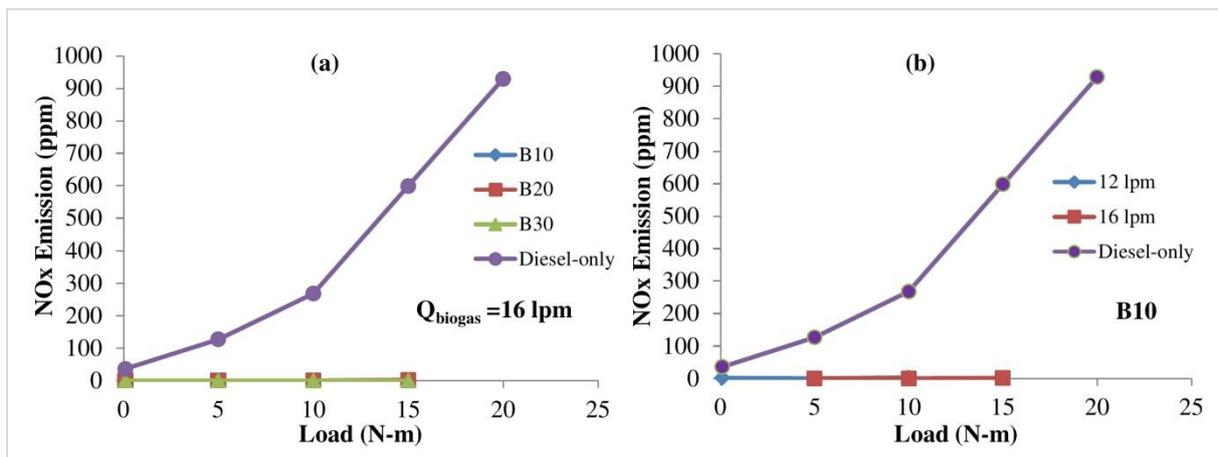
Figure 6: Effect of (a) butanol blending ratio and (b) biogas flow rate on NO<sub>x</sub> emission
