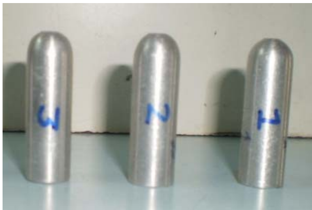
Fig .1: Al-SiC-Flyash metal matrix samples used for standard for Wear Test
