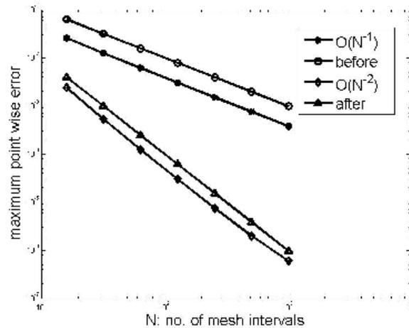
Fig. 3. Comparison of nodal errors on adaptive grid.
