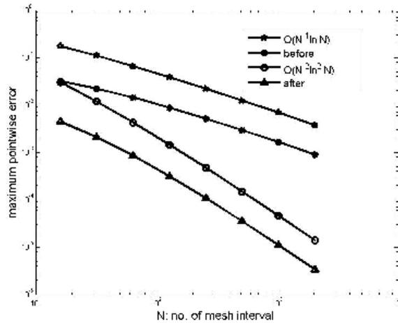
Fig. 1. Comparison of nodal errors on S-mesh.
