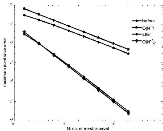
Fig. 2. Comparison of nodal errors on B-S-mesh.
