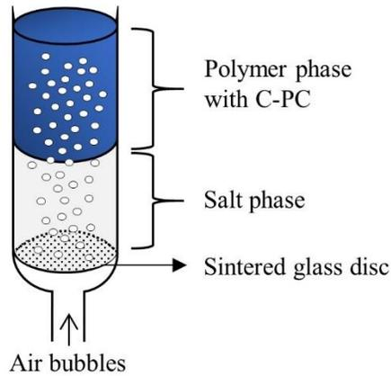
Figure 1: Schematic diagram of the PEG/salt-based LBF for the purification of phycocyanin from *Spirulina*. The flotation effects created with the air bubbles assist in the upwards flow of phycocyanin from the bottom aqueous salt solution to the PEG-rich top phase.
