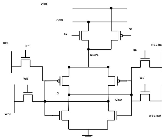
**Figure 4 (a).** MCPL based SRAM Cell with Read and Write access transistors
