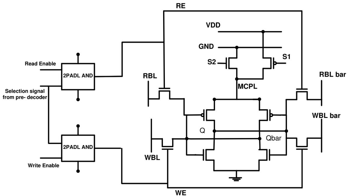
**Figure 7 (a)** MCPL Based SRAM Cell with 2PADL auxiliary circuits.
