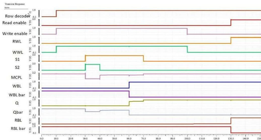
**Figure 4. (b)** MCPL based SRAM Cell with Read and Write Operation
