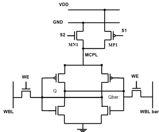
**Figure 2.** SRAM Cell with MCPL
