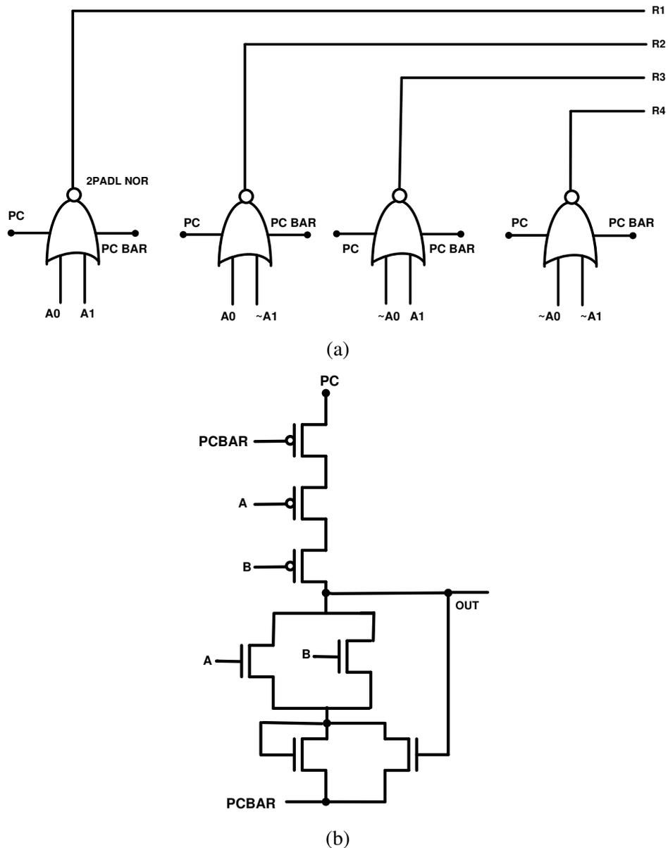
**Figure 6.** (a) 2PADL Pre-Decoder (b) Transistor Schematic of 2PADL NOR
