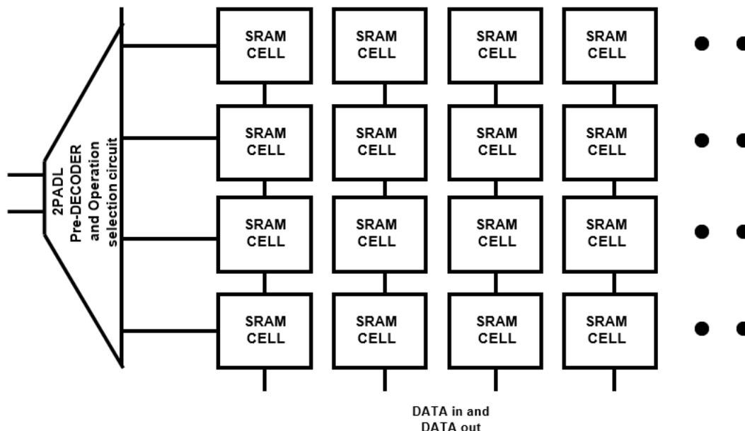
**Figure 5.** Architecture of SRAM Array
