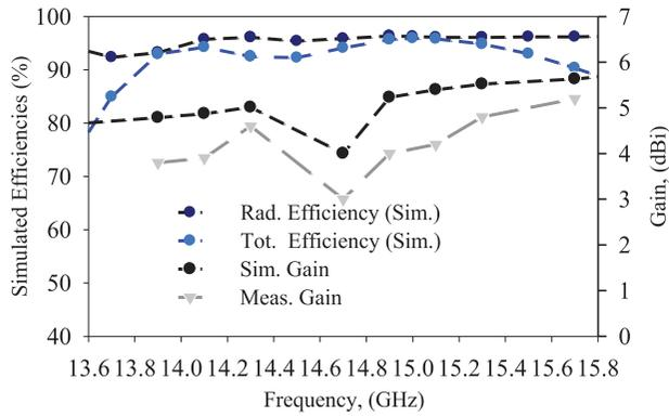
**Figure 11:** The antenna efficiencies and radiation gain performance
