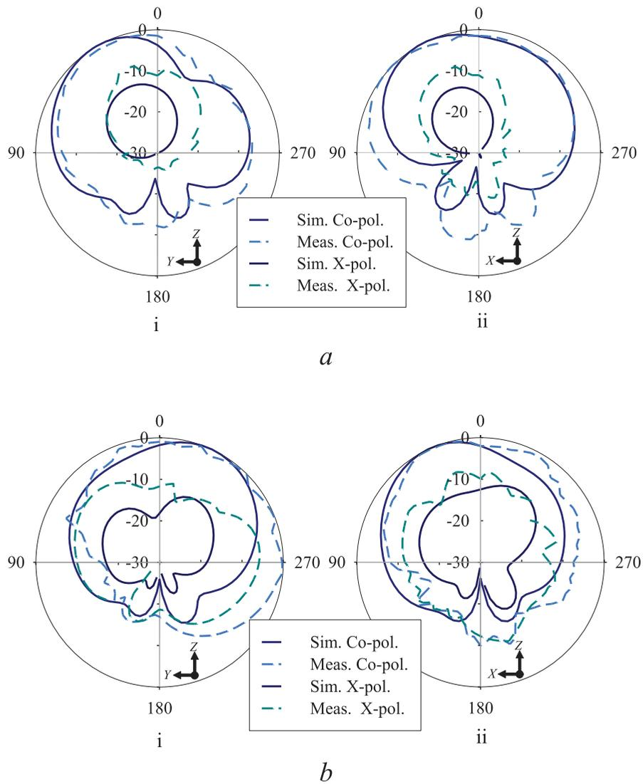
**Figure 12:** Radiation Profiles at: (a) 13.8 GHz: (i) yz-plane and (ii) xz-plane and (b) 15 GHz: (i) yz-plane and (ii) xz-plane.
