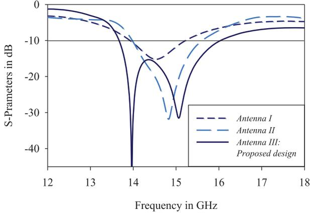
**Figure 3:** S-parameter response for design evolution
