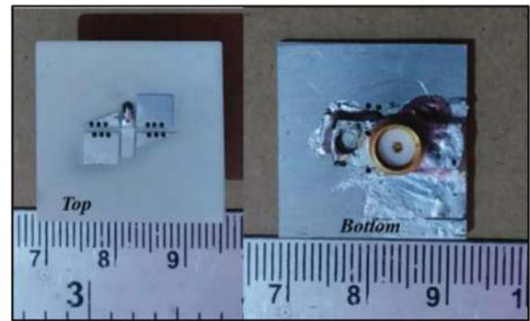
Figure 9: The top and bottom view of the fabricated antenna prototype
