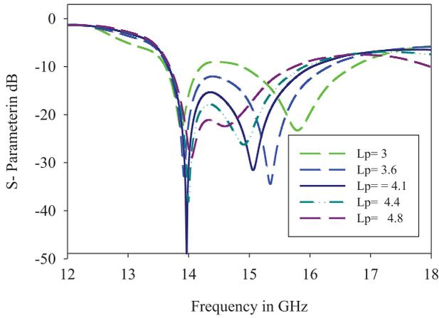
Figure 5: The S-parameters: variation in parameter " $L_p$ "
