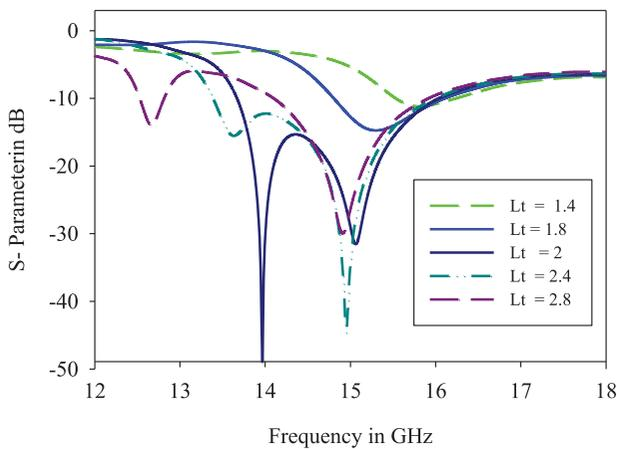
Figure 7: The S-parameters: variation in parameter " $L_t$ "
