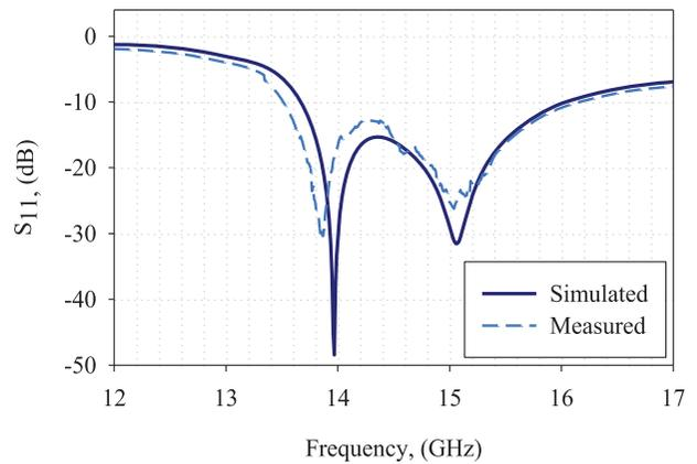
Figure 10: Simulated and measured reflection coefficients ( $S_{11}$ )
