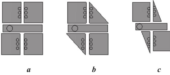
**Figure 2:** The design evolution of the proposed antenna. (a) Antenna I: with rectangular patches, (b) Antenna II: with truncated rectangular patches, and (c) Antenna III: the proposed design
