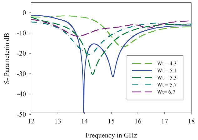
Figure 8: The S-parameters: variation in parameter " $W_t$ "
