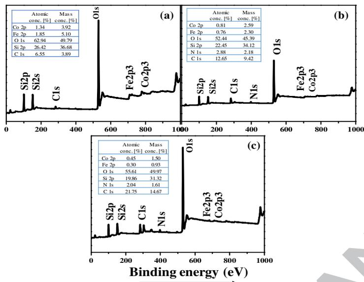
**Fig. 7.** Full scan XPS spectra of (a)  $\text{SiO}_2@CoFe_2O_4$ , (b)  $\text{SiO}_2@CoFe_2O_4-NH_2$  and (c) amino-functionalized  $\text{SiO}_2@CoFe_2O_4-GO$  nanocomposites.
