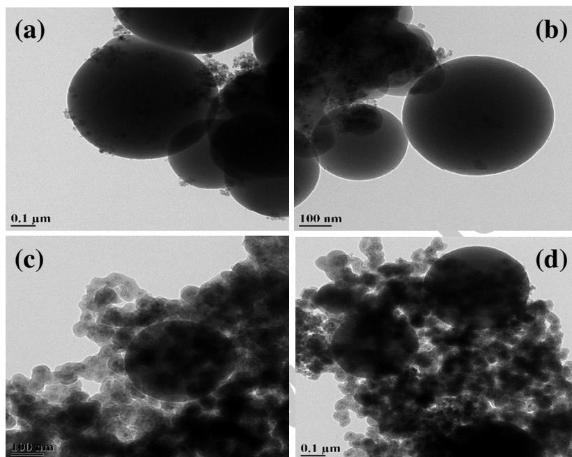
**Fig. 4.** HR-TEM images of (a)  $\text{SiO}_2@\text{CoFe}_2\text{O}_4$ , (b)  $\text{SiO}_2@\text{CoFe}_2\text{O}_4\text{-NH}_2$ , (c-d) amino-functionalized  $\text{SiO}_2@\text{CoFe}_2\text{O}_4\text{-GO}$ .
