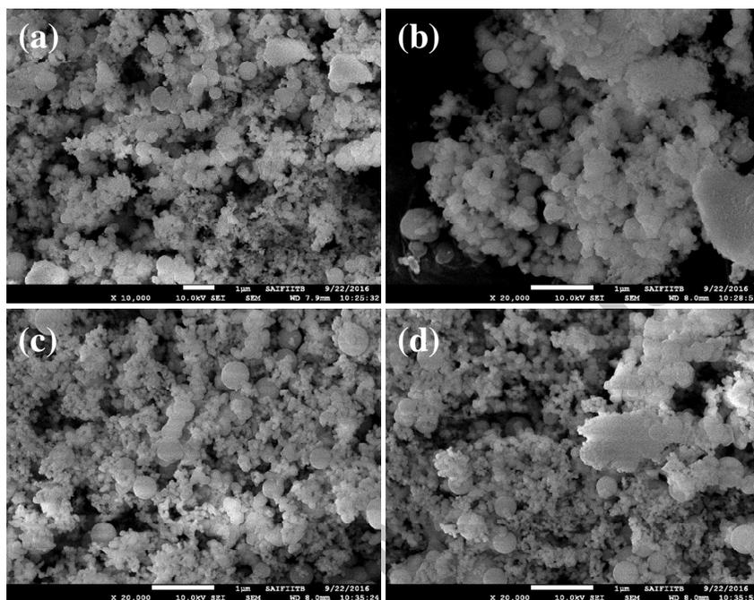
**Fig. 3.** FE-SEM images of (a) SiO<sub>2</sub>@CoFe<sub>2</sub>O<sub>4</sub>, (b) SiO<sub>2</sub>@CoFe<sub>2</sub>O<sub>4</sub>-NH<sub>2</sub>, (c-d) amino-functionalized SiO<sub>2</sub>@CoFe<sub>2</sub>O<sub>4</sub>-GO.
