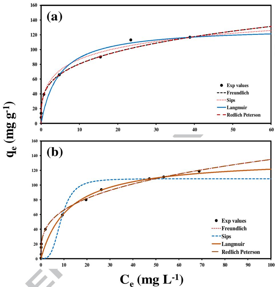
**Fig. 12.** Adsorption isotherms of (a) AB 1 and (b) Cr(VI) by amino-functionalized  $\text{SiO}_2@CoFe_2O_4$ -GO nanocomposites and fitting of different isotherm models to the experimental data. (Contact time: 140 min, pH 1 for Cr(VI) ions and pH 2 for AB 1, adsorbent dosage:  $0.5 \text{ g L}^{-1}$ , temp:  $25^\circ\text{C}$ )
