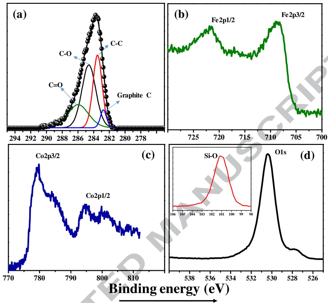
**Fig. 8.** XPS spectra of (a) C1s (b) Fe2p (c) Co2p and (d) O1s (Inset shows SiO<sub>2</sub>) regions of amino-functionalized SiO<sub>2</sub>@CoFe<sub>2</sub>O<sub>4</sub>-GO nanocomposites.
