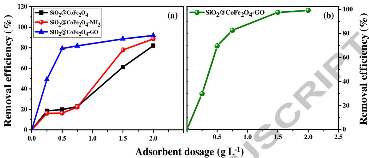
**Fig. 9.** Effect of adsorbent dosage on (a) AB 1 adsorption by synthesized nanocomposites, (b) Cr(VI) ions adsorption by amino-functionalized SiO<sub>2</sub>@CoFe<sub>2</sub>O<sub>4</sub>-GO nanocomposites. (Contact time: 140 min, pH 1 for Cr(VI) ions and pH 2 for AB 1, initial concentration: 10 mg L<sup>-1</sup>, temp: 25°C)
