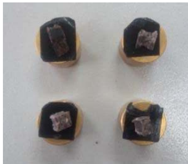
Figure 1. Samples for Scanning Electron Microscopy (SEM).
