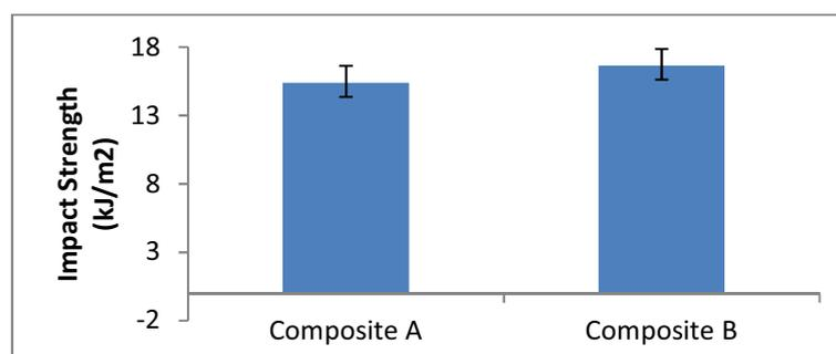
**Figure 7.** Impact strength of Composite A and B
