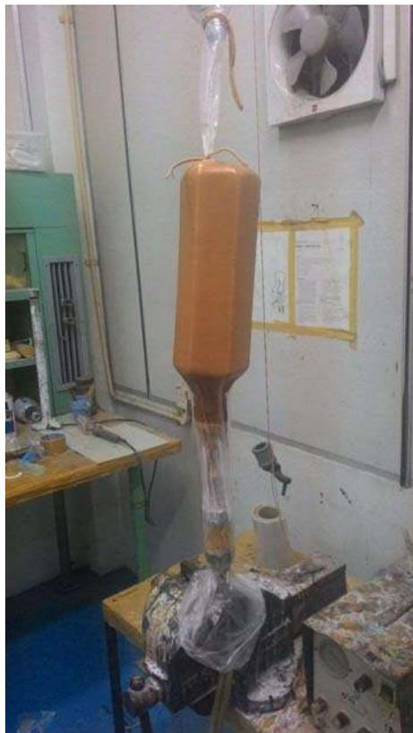
**Figure 1.** The laminated of woven kenaf composite in hexagon mould using vacuum infusion.
