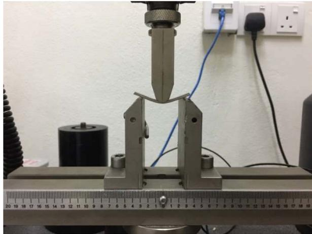
Figure 3. Flexural specimen tests
