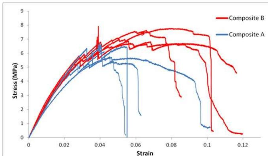
**Figure 4.** The flexural stress versus strain curves for composites A and B.
