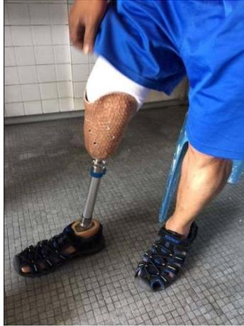
**Figure 8.** Patient donning the prosthetic socket made from kenaf woven fabric composite
