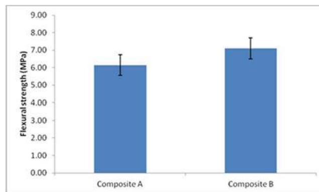
**Figure 6.** Flexural strength of Composite A and B
