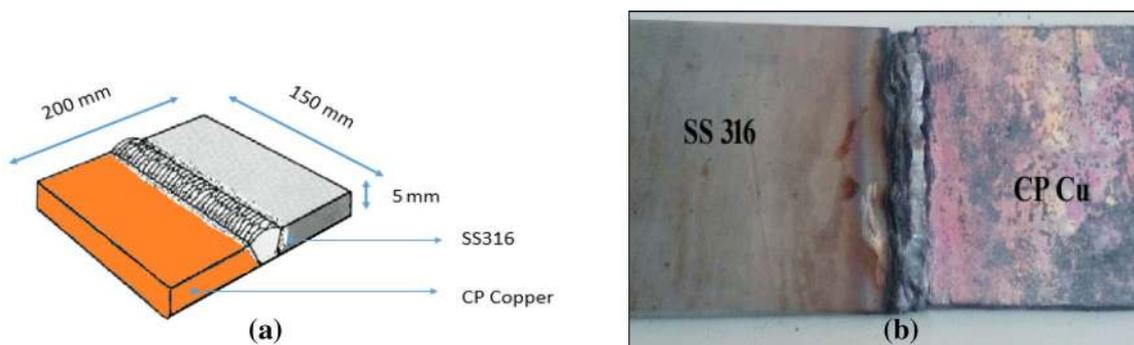
**Fig. 1** (a) Schematic dimension of weld plates and (b) plates after TIG welding
