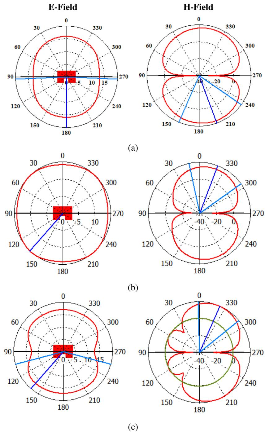
**Figure 5.** E-field and H-field radiation patterns of WSP antenna at (a) 6.97 GHz, (b) 10.12GHz, (c) 15.78GHz frequencies
