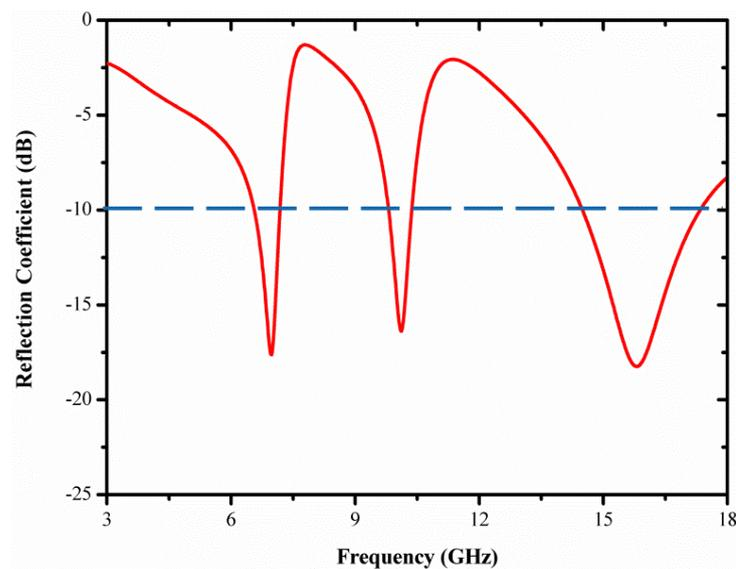
**Figure 7.** S11 of conformal WSP antenna mounted on a missile.
