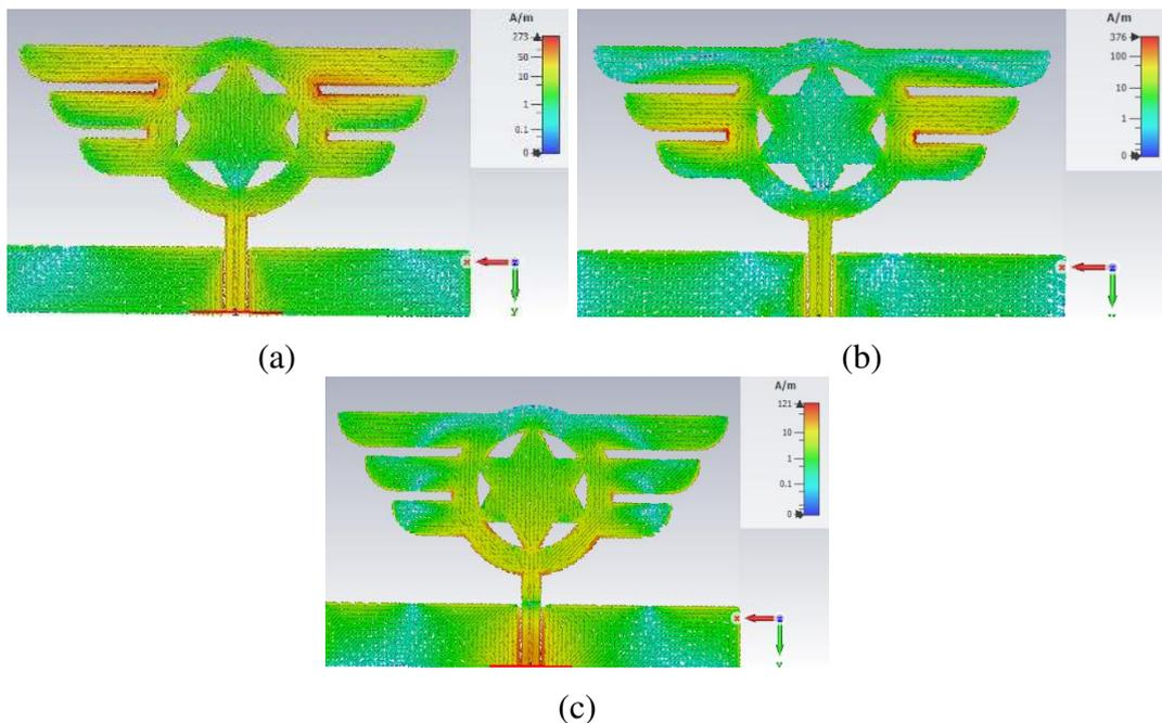
**Figure 4.** Surface current distribution of WSP antenna at (a) 6.97 GHz, (b) 10.12GHz, (c) 15.78GHz frequencies.
