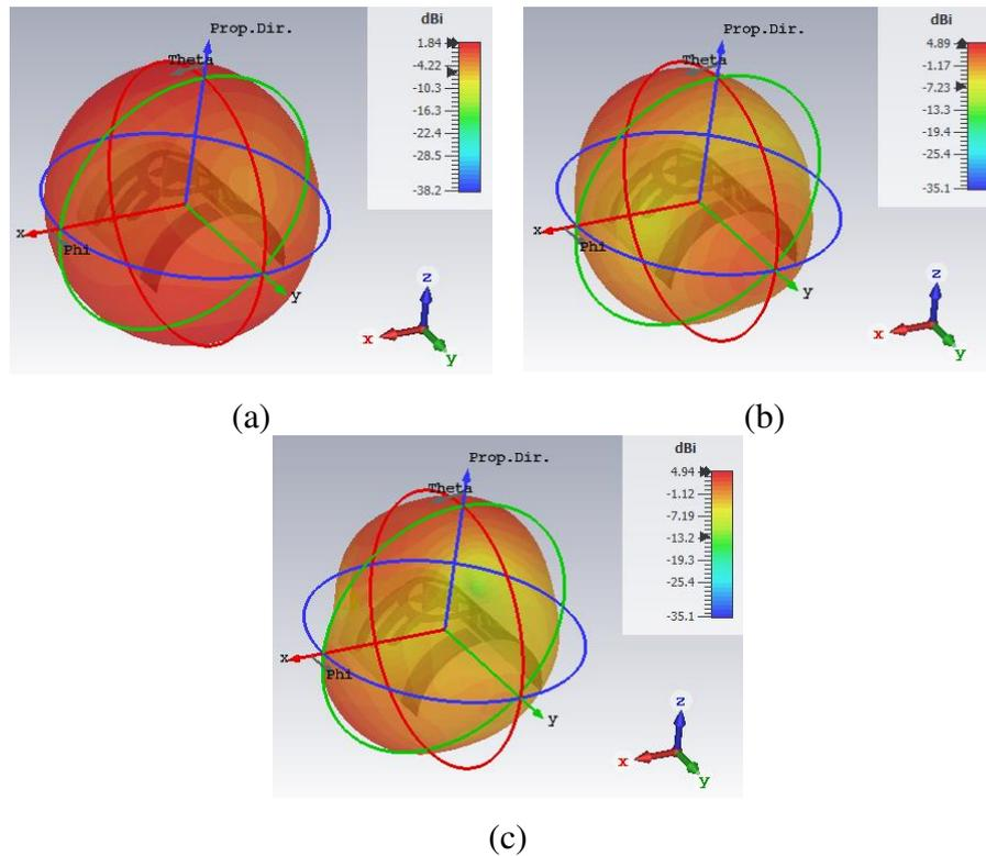
**Figure 8.** 3D-Gain plot of conformal WSP antenna at (a) 7 GHz, (b) 10.24GHz, (c) 16.16GHz frequencies.
