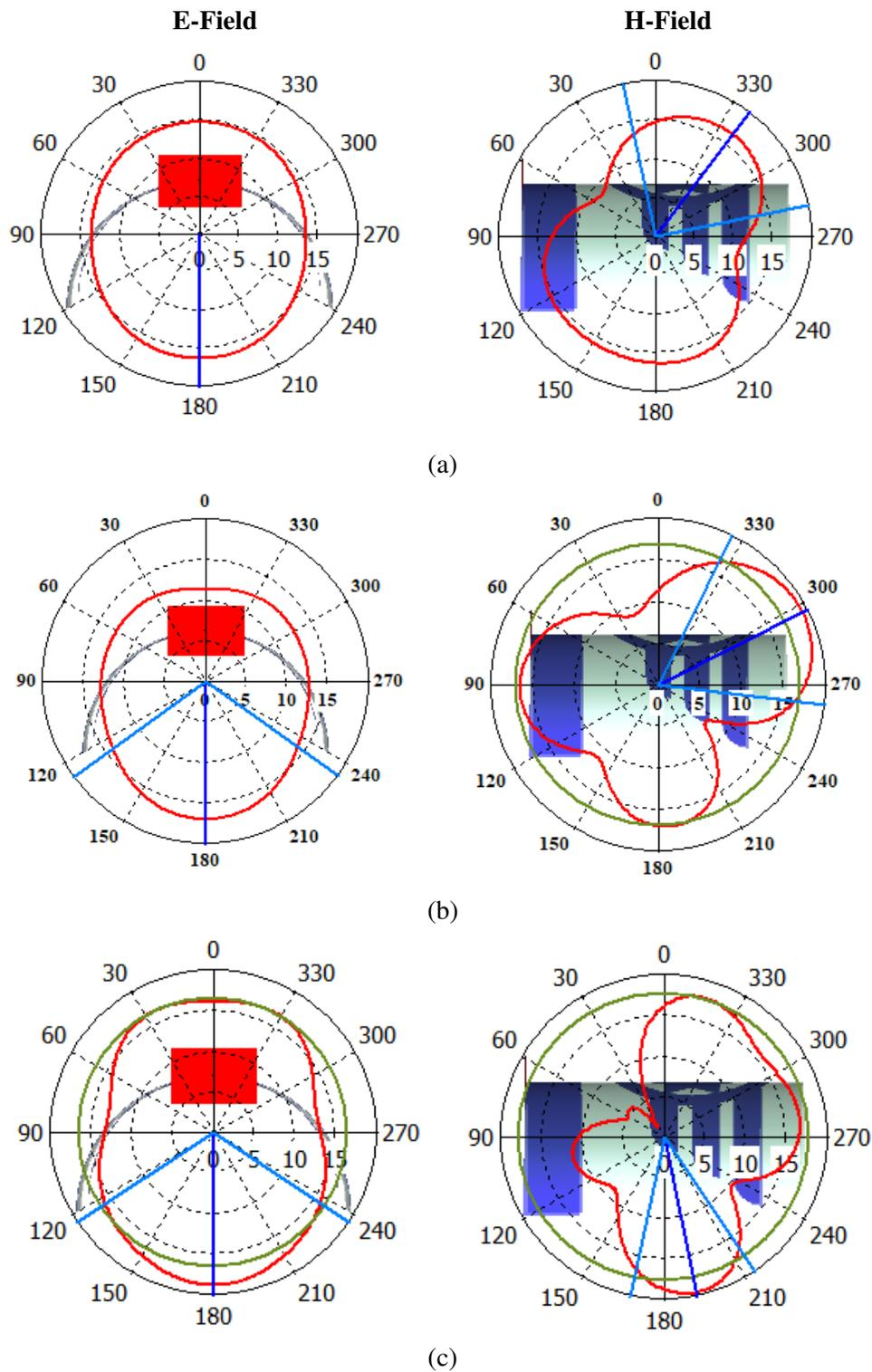
**Figure 9.** E-field and H-field radiation patterns of conformal WSP antenna (a) 7 GHz, (b) 10.24GHz, (c) 16.16GHz frequencies.
