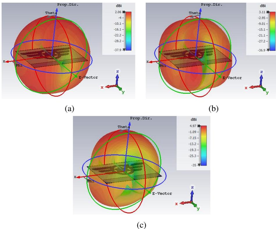
Figure 3. 3D-Gain plot of proposed wing-shaped patch (WSP) antenna at (a) 6.97 GHz, (b) 10.12GHz, (c) 15.78GHz frequencies.
