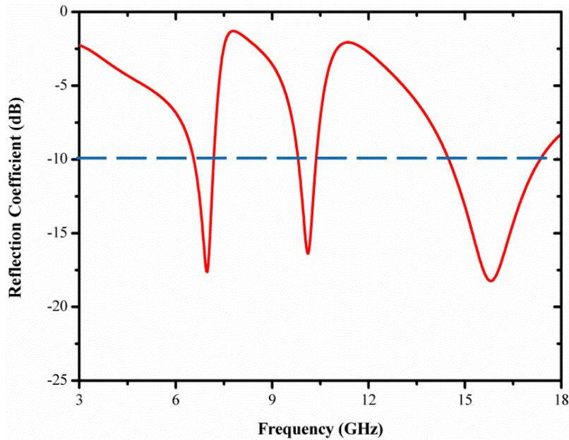
Figure 2.  $S_{11}$  of wing-shaped patch (WSP) antenna.
