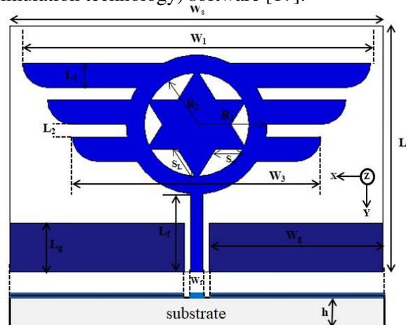
**Figure 1.** The geometry of the wing-shaped patch (WSP) antenna.
