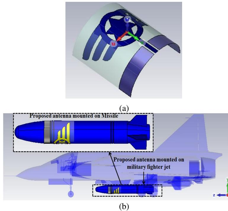
**Figure 6.** The geometry of (a) conformal WSP antenna, (b) WSP antenna mounted on aircraft with a guided missile.
