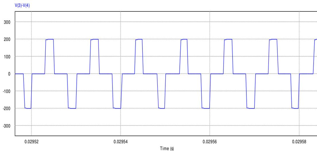
**Figure 6.** Output voltage at transformers secondary terminal
