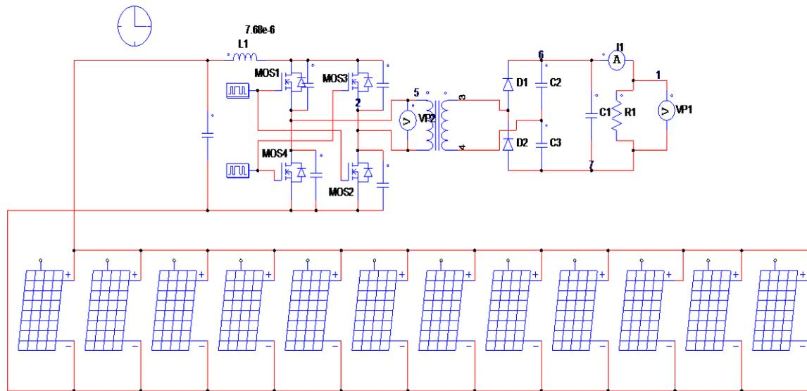
**Figure 1.** A Current Fed DC-DC Converter topology with voltage doubler rectifier in the output
