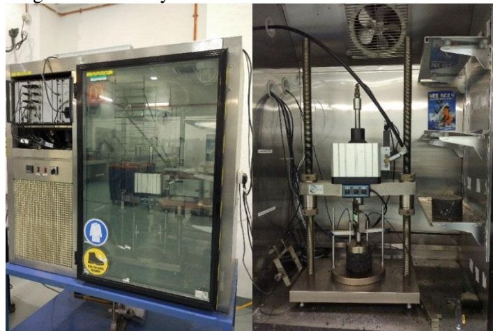
Fig 3. Universal Testing Machine, UTM-5P
