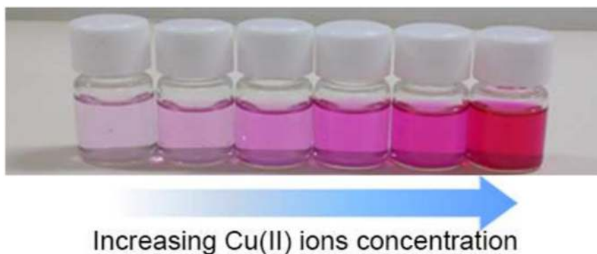
Fig. 14. Linear increase in color concentration with increase in concentration of \text{Cu}^{2+} ions. (Reproduced with permission) [100].
